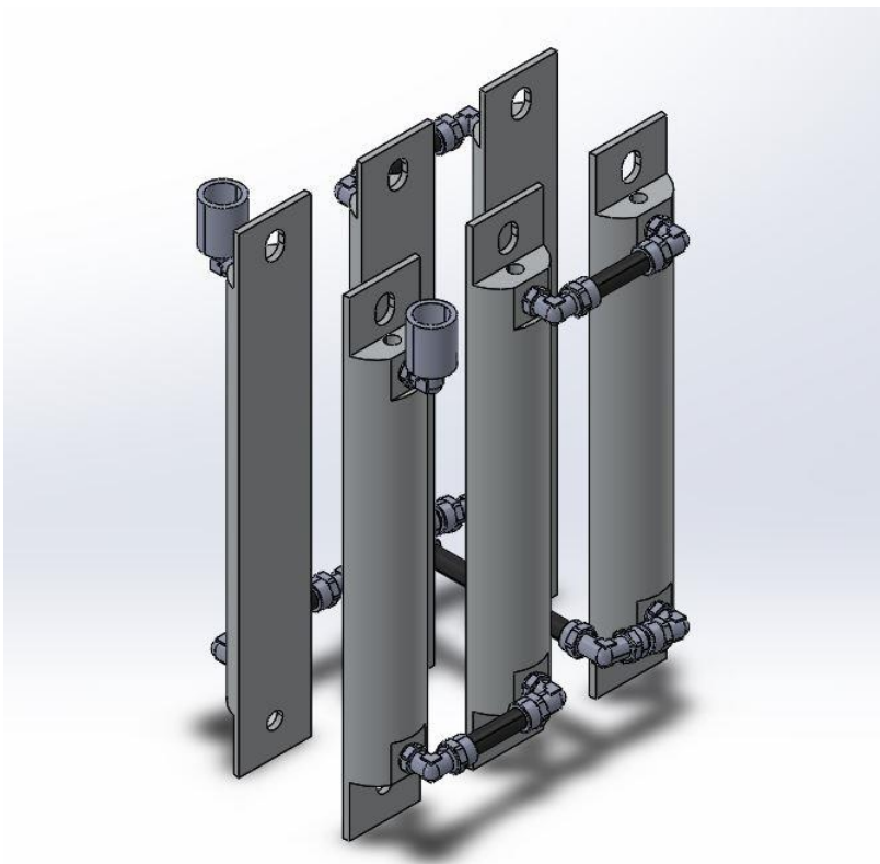
Figure 3.4.4.3.8 Choke MS14813 cooling contour in three-dimensional view
