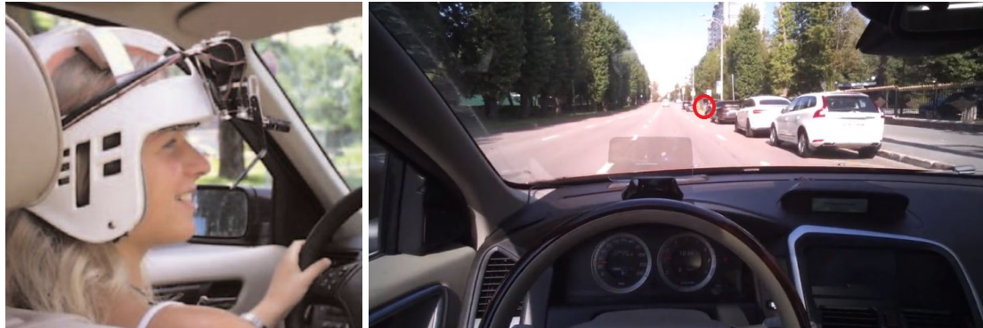
Figure 5: Eye tracking system. Source HUDWAY youtube video and EYE GAZE STUDIES, Munich
