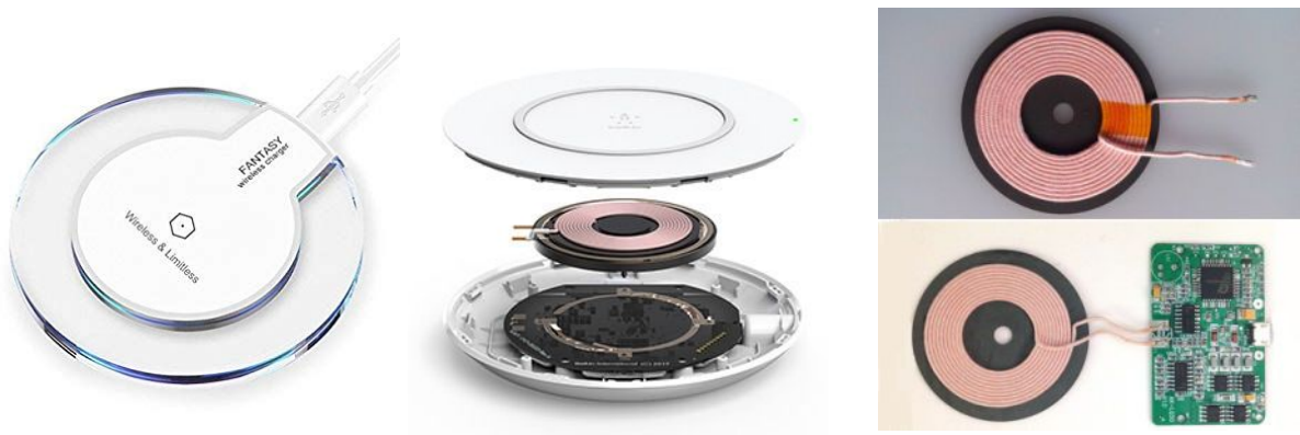
Figure 27: Pictures of wireless charger and inductive coil (source www.amazon.co.uk )
