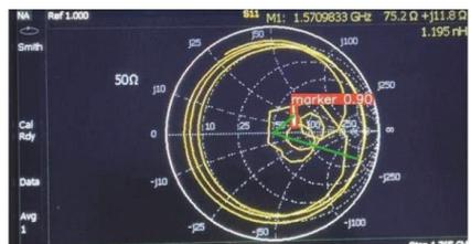
Fig. 8. Marker tracking when last screw is tuned
