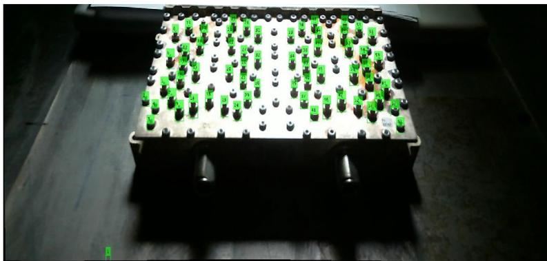
Figure 6.7. Tuning screws predicted by KNN model (also published in [VI])
