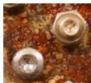
Figure 6.9. Different types of tuning screws on a cavity filter (also published in [IV])
