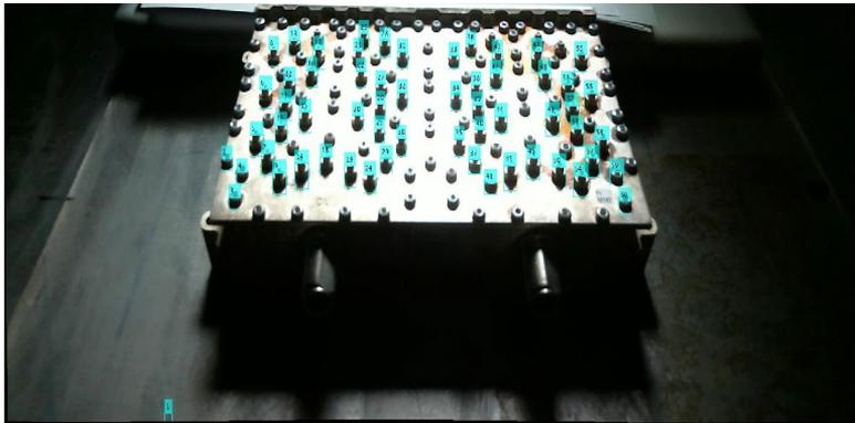
Figure 6.6. Tuning screws predicted by SVM model (also published in [VI])
