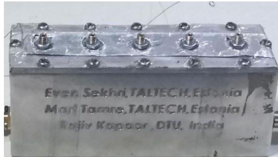
Figure 7.7. A thin metallic sheet on the filter's top plate to implement the nut locking strategy.
