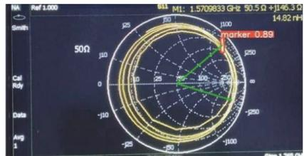
Fig. 7. Marker being tracked while tuning the first screw is getting tuned
