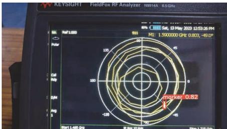
Fig. 9. Tracking the tuning parameters in polar plot without implementing the preprocessing block presented in Fig 3.
