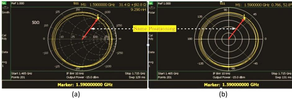
Figure 7.3. Keysight 9914A VNA's Smith chart (left) and Polar display (right)
