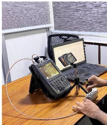
Figure 7.12. Generation of dataset while filter is being tuned manually
