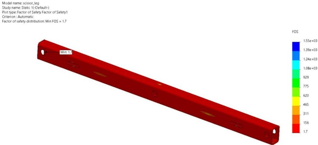
Figure 5.9.4 Factor of safety for scissor link
