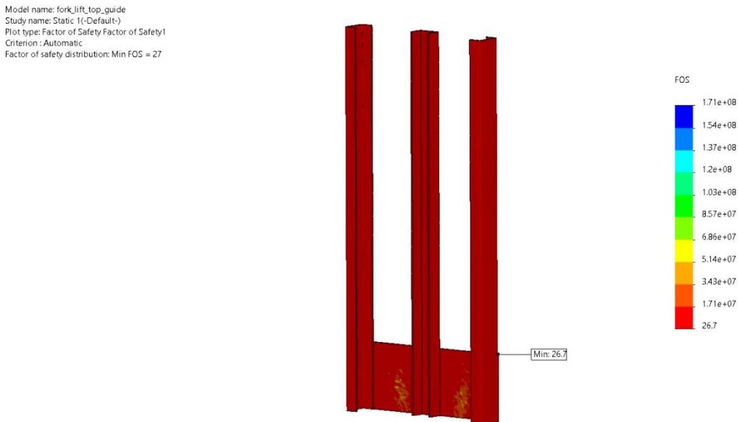
Figure 5.5.5 Factor of safety of the forklift drive guide
