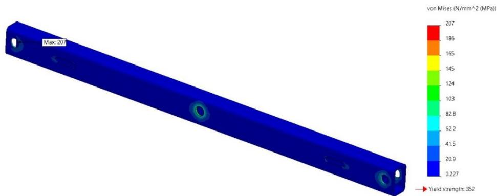
Figure 5.9.1 Stress of scissor link
