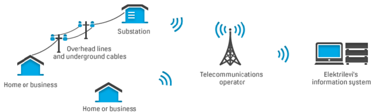
Figure 3.6 Remotely read meters work [40]
