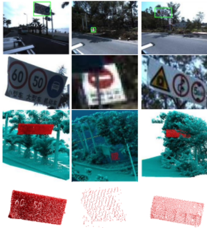
Figure 3. Traffic sign damage analysis using image MLS data [10]
