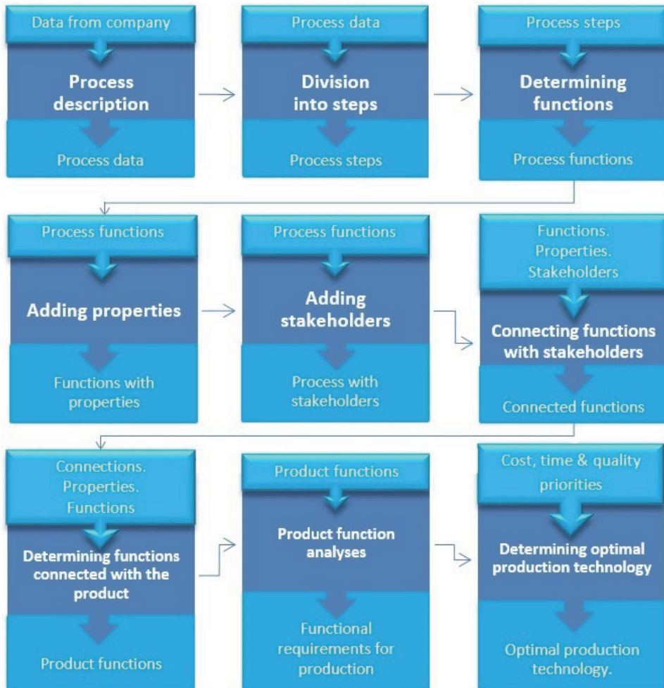
Figure 2.1 Inputs and outputs for each step for creating a FR model. The inputs are at the top of each step, the outputs at the bottom.
