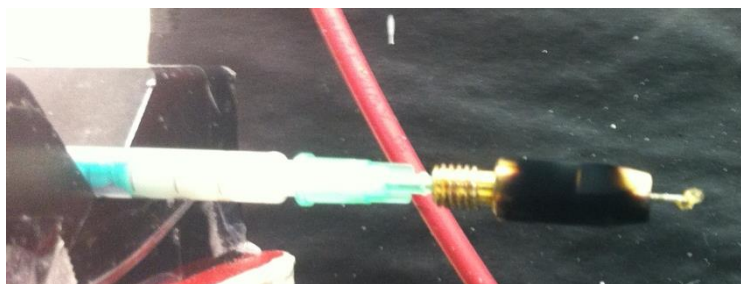
Figure 6. Needle with copper cylinder (with central hole of 0.8 mm)
