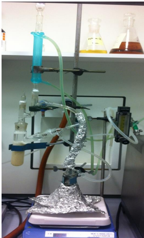
Figure 8. Soxhlet extractor setup (with 100ml of methanol at 125°C)
