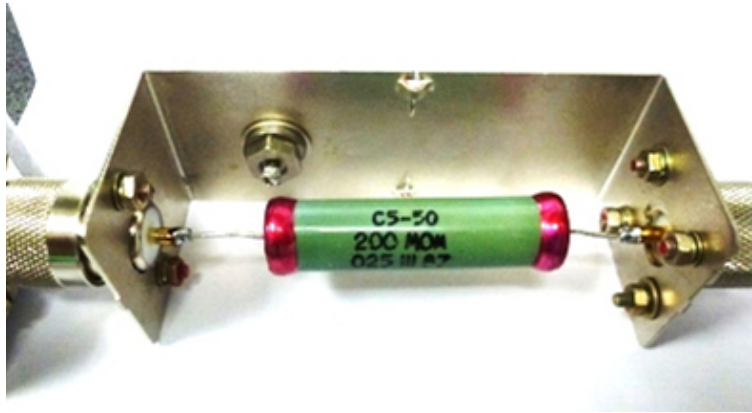
Figure 3.8: Wire wound resistor with the nominal impedance of 200\text{ M}\Omega
