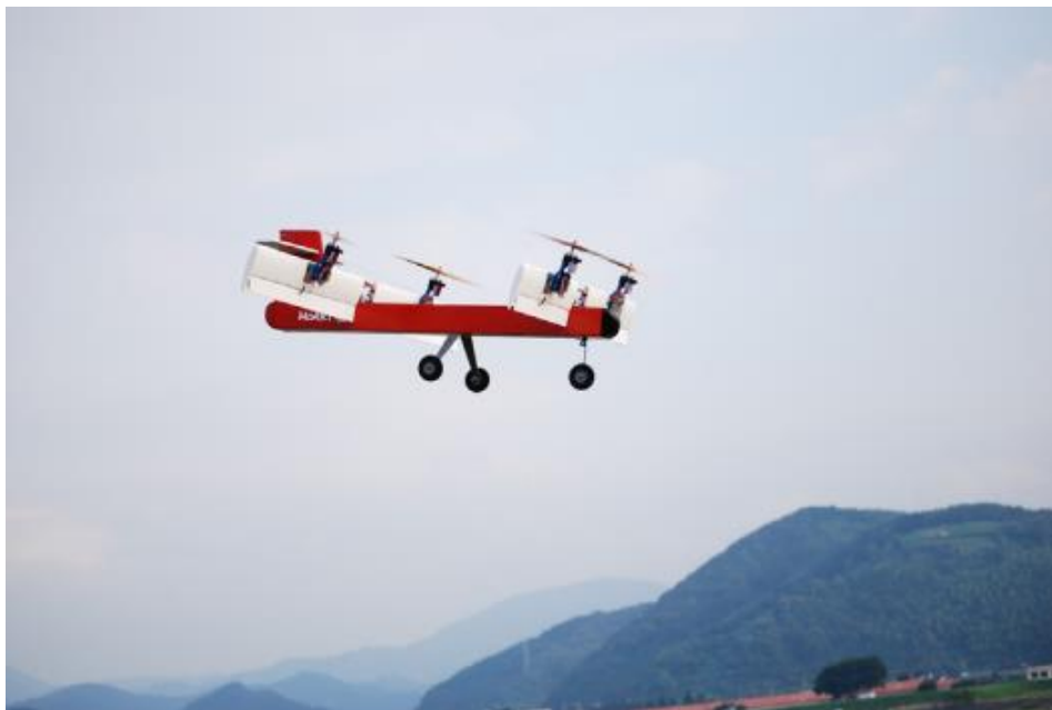
Figure 2.5 Accelerating transition of a tiltwing VTOL with 2 pair of wings [21]
