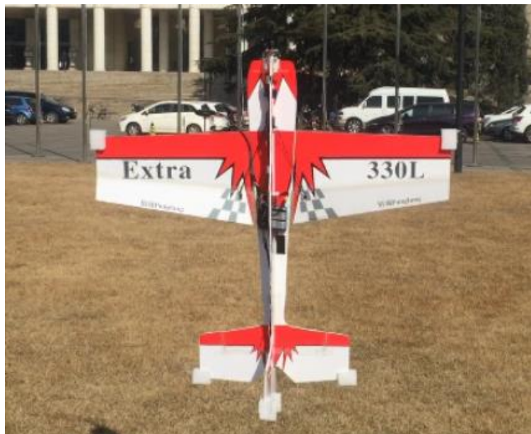
Figure 2.1 Tail-sitter with a Single Thrust-Vector Propeller [6]
