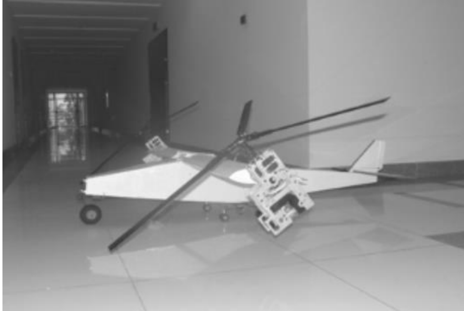
Figure 2.4 Experimental tiltrotor aircraft with 2 propellers on the wings [16]
