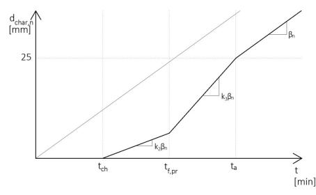
Figure 3.4 Determination of charring depth with time when  $t_{ch} < t_{f.}$  Reference line is charring of initially unprotected member. [10]
