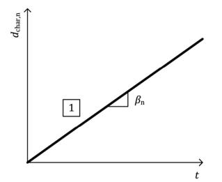
Figure 4.1 Charring depth of initially unprotected member: 1 – normal charring phase (phase 1), t – time,  $d_{char,n}$  – notional charring depth,  $\beta_n$  – notional charring rate.
