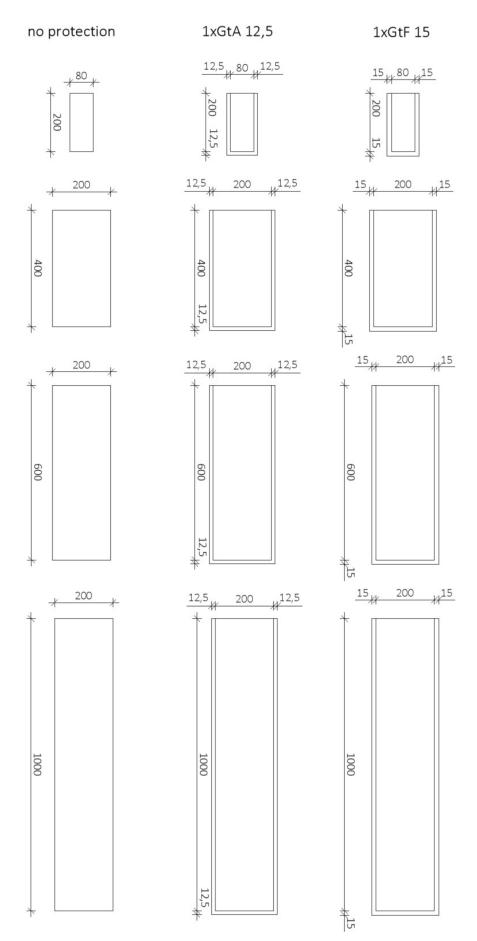
Figure 1.2 Cross-sections of beams used in this thesis
