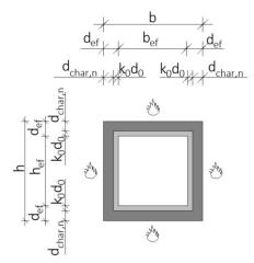
Figure 3.6 Effective cross-section for columns
