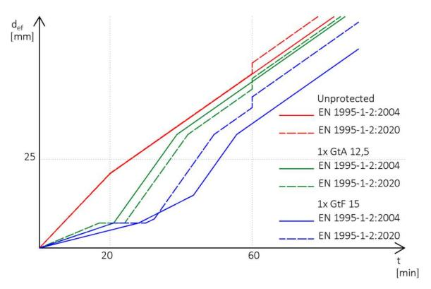
Figure 6.3 The change of the effective depth of the char layer on beams over time,  $d_{ef}$  – effective charring depth.
