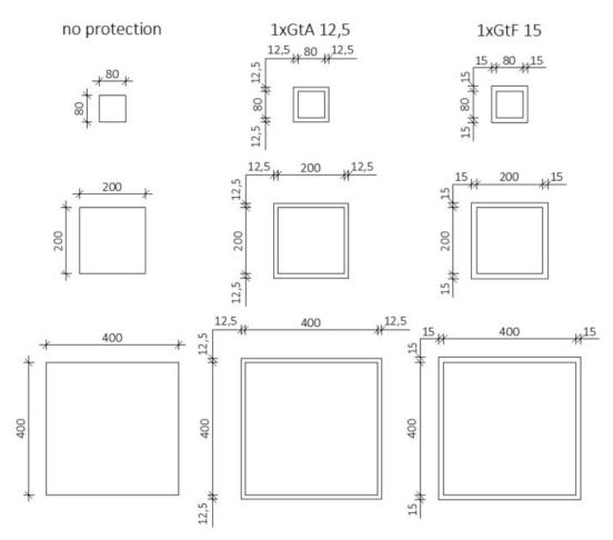
Figure 1.3 Cross-sections of columns used in this thesis
