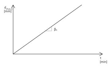
Figure 3.1 Relationship for initially unprotected members throughout the time of fire exposure [10]
