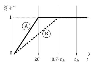
Figure 4.5 Determination of the value of zero-strength layer depth  $d_0$  as a function of the time, A – increase of the zero-strength layer depth for initially unprotected members, B – increase of the zero-strength layer depth for initially protected members
