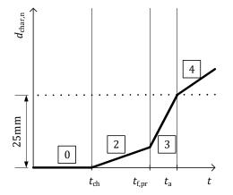
Figure 4.4 Charring of initially protected sides of timber members when  $t_{f,pr}>t_{ch}$  [6]
