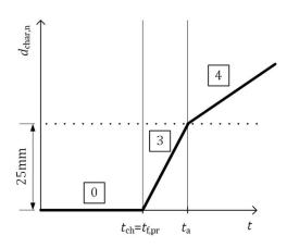
Figure 4.2 Charring of initially protected sides of timber members when  $t_{f,pr}=t_{ch}$  and the charring depth at  $t_a$  is 25 mm [6]
