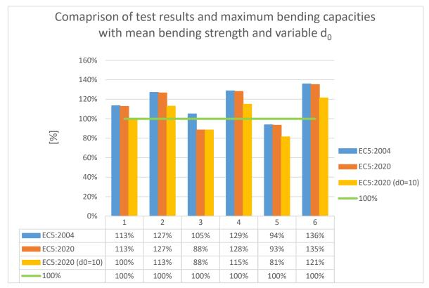
Figure 7.3 Comparison of test results and maximum bending capacities with mean bending strength and variable  $d_{0} \end{tabular}$
