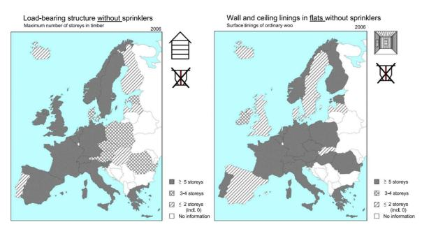
Figure 1.1 Restricted use of load-bearing timber structures and visible wood set by national prescriptive regulations [2]
