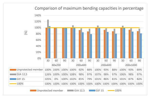
Figure 6.1 Comparison of maximum bending capacities on beams in percentage
