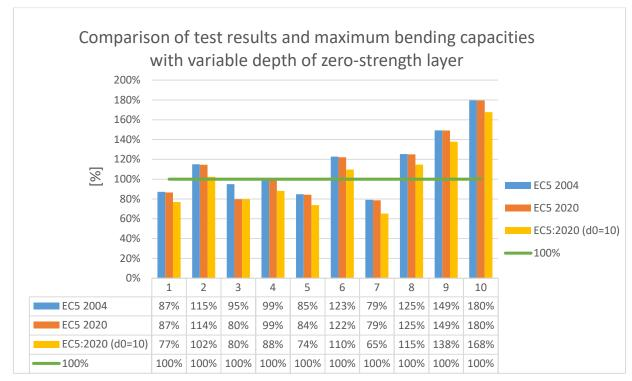
Figure 7.2 Comparison of test results and maximum bending capacities with variable d<sub>0</sub>
