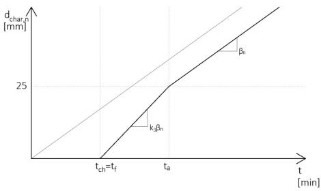
Figure 3.2 Determination of charring depth with time when  $t_{ch}=t_f$  and the charring depth at time  $t_a$  is at least 25 mm. Reference line is charring of initially unprotected member. [10]
