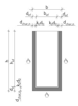
Figure 3.5 Effective cross-section for beams
