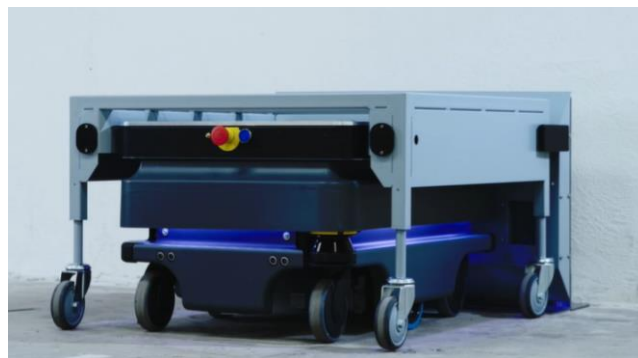
Figure 28. Custom cart design for AMR MIR250 [36]
