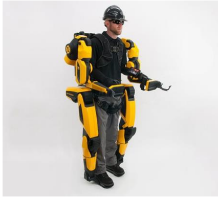
Figure 2.4 Full body exoskeleton Guardian XO of Sarcos Robotics [13]
