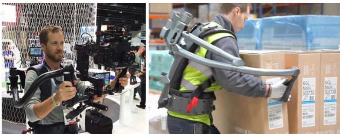
Figure 2.2 Exhaus upper body exoskeletons in work [10]
