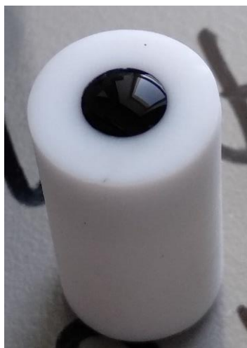
Fig. 2.3. Catalyst ink deposited to the electrode surface for RDE test
