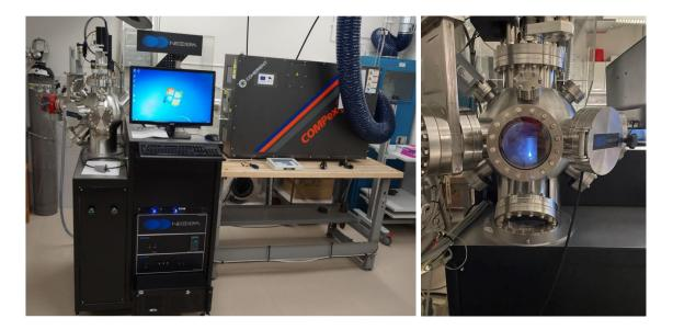
Figure 11 Pulsed laser deposition system Neocera Pioneer 120
