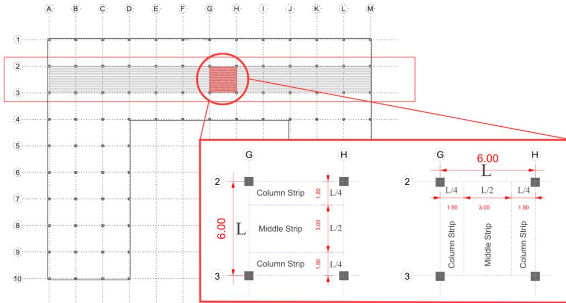
Figure 4.9. Slab span details and Eurocode 2 slab design considerations for a sample 6-meter bay width
