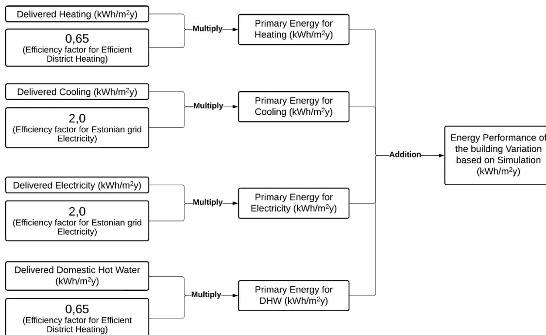
Figure 4.22. Flow chart of the methodology of the calculations of primary energy demand and energy performance of building variations based on simulations
