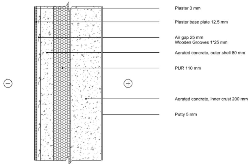
Figure 4.17. Details of layers of Autoclaved Aerated Concrete Walls (V3)
