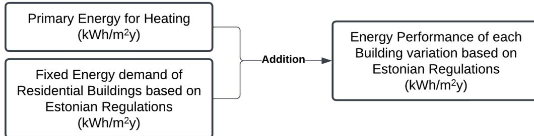
Figure 4.23. Methodology of calculating building variations energy performance based on Estonian Regulations for residential buildings
