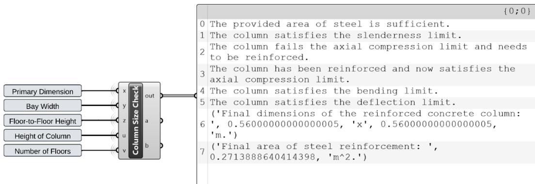
Figure 4.12. An illustration of column designer component inside Grasshopper
