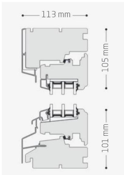
Figure 4.14. Details of window profile
