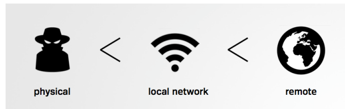
Figure 3. "physical" include data extraction from onboard memory chip or direct serial communication to the board. "local network" means intercepting wireless communications. "remote" is port scanning or more further trial from remote site [4]
