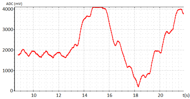
Fig. 1.6. Medical radar output waveform. Measured with 12-bit ADC from a distance of 90 cm. Breath is held in the beginning, followed by one deep respiratory cycle.
