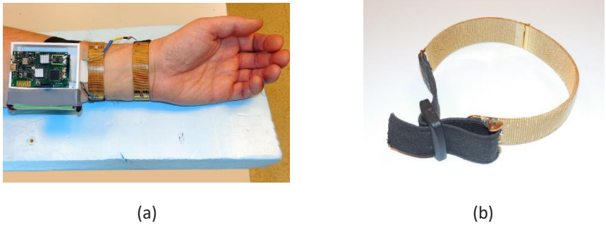
Fig. 4.24 Measurement of the forearm impedance at a distance of 4 cm (a) and used flexible capacitive electrode (b).
