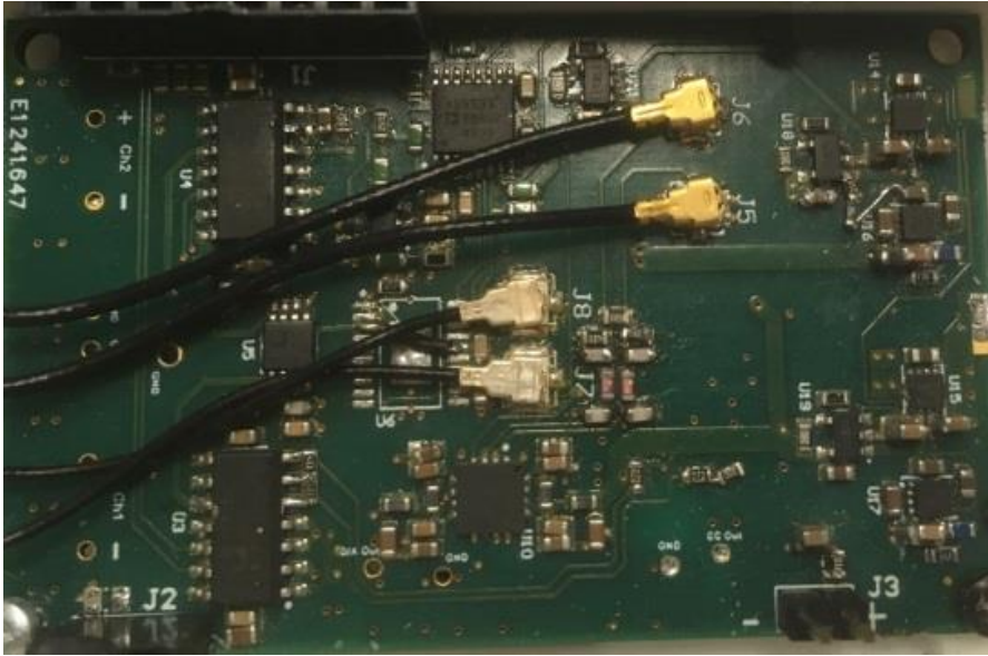
Fig. 4.5 Compact Impedance Analyzer analog board.
