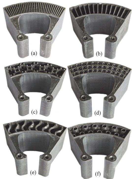
FIGURE 5. AM heatsink sectors: a) conventional straight fins, b) airfoil pin fins, c) rhombi octet, d) BCC e) TPMS gyroid, f) TPMS diamond.
