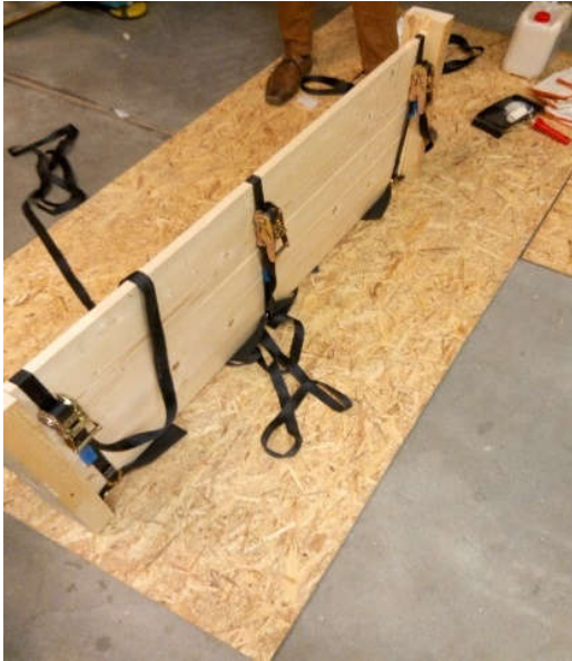
Figure 3.1. Setup used for gluing lamellas edge-to-edge.
