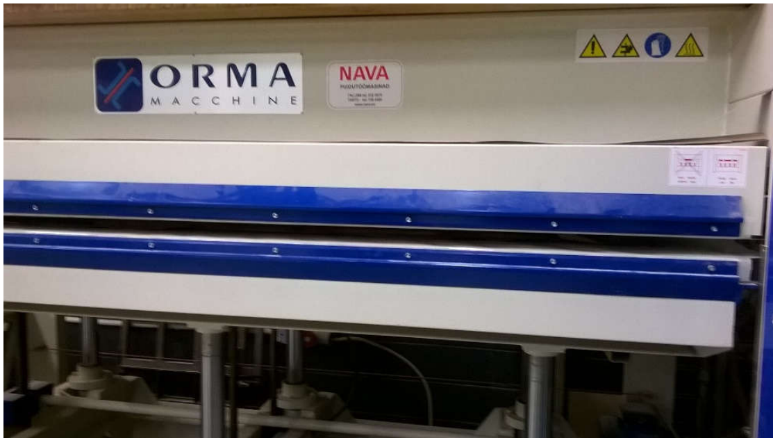
Figure 3.5. Cold press equipment.
