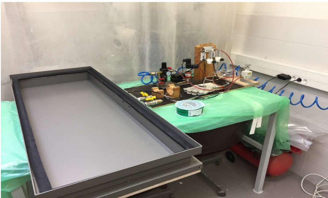
Figure 3.10. Air permeability box and remaining test apparatus.
