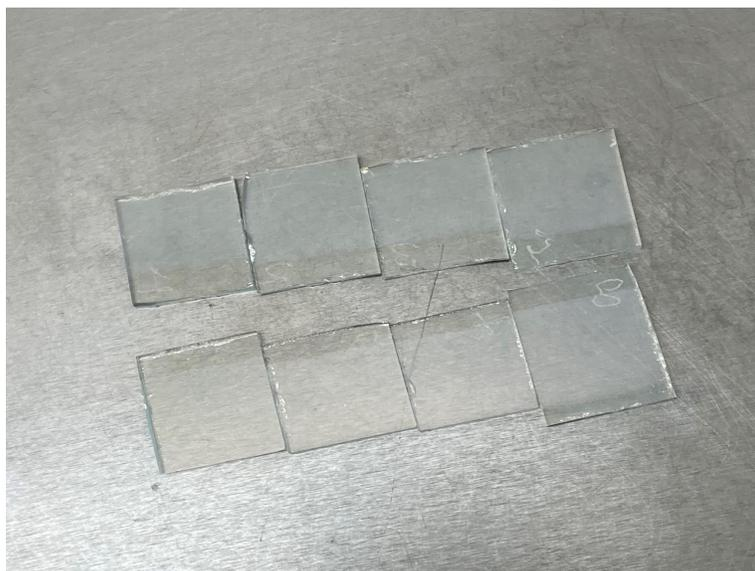
**Figure 18.** TiO<sub>2</sub> deposited and annealed samples on glass/FTO substrate.
