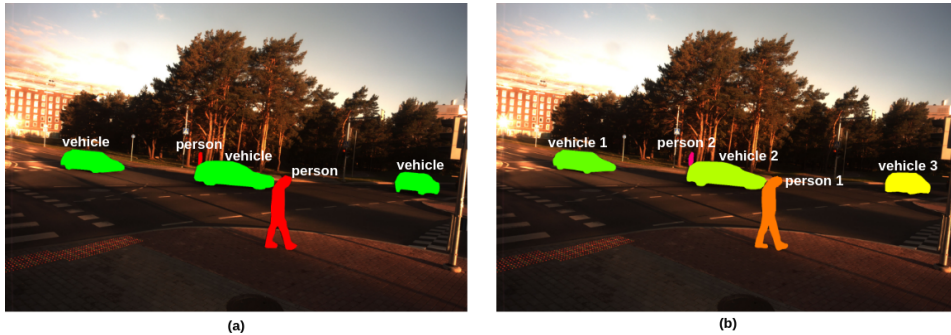
Figure 1: Examples of semantic and instance segmentation. (a) is the semantic segmentation, where objects of the same class are highlighted by the same color. (b) is the instance segmentation, where each object from the same class is assigned by an individual color. The sample image is from the custom iseAuto dataset [24].
