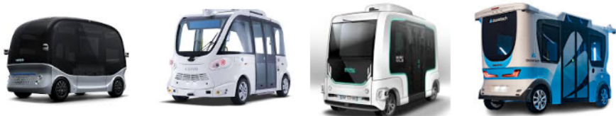
Figure 2: Illustrations of several commercial autonomous shuttles. From left to right are Apollo Minibus [103], Navya Evo [104], Easymile EZ10 [105], and AuveTech MiCa [106].
