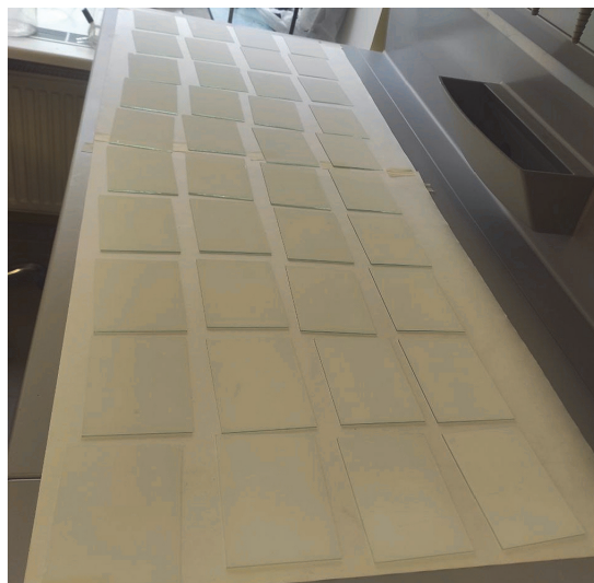
Fig. 4. Glass plates covered with TiO 2 by spraying.
