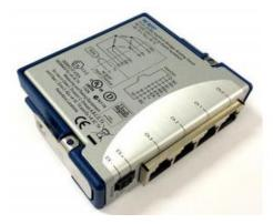
Figure 6.9 NI 9237 DAQ Board [34]
