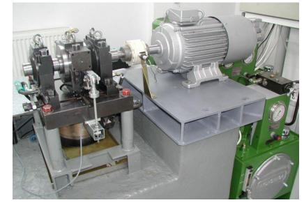
Figure 4.2 PG-2 1Ł - test rig for journal bearings [10]
