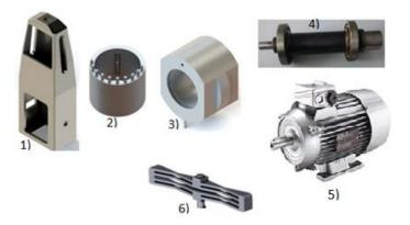
Figure 2.4, 1) Bearing housing, 2) Inner Bearing, 3) The existing outer bearing, 4) The existing bearing shaft, 5) motor [16], 6) The existing load gauge
