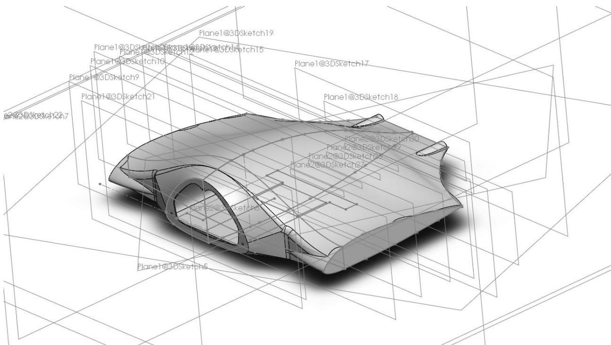
Figure 5.7: Full body of the drone.
