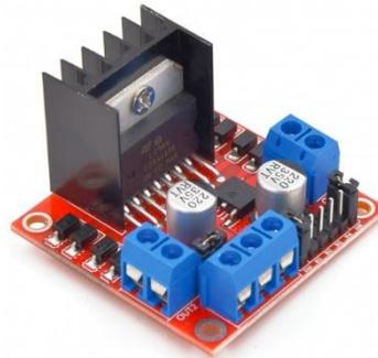
Figure 0.5: L298N chipset based motor driver board.
