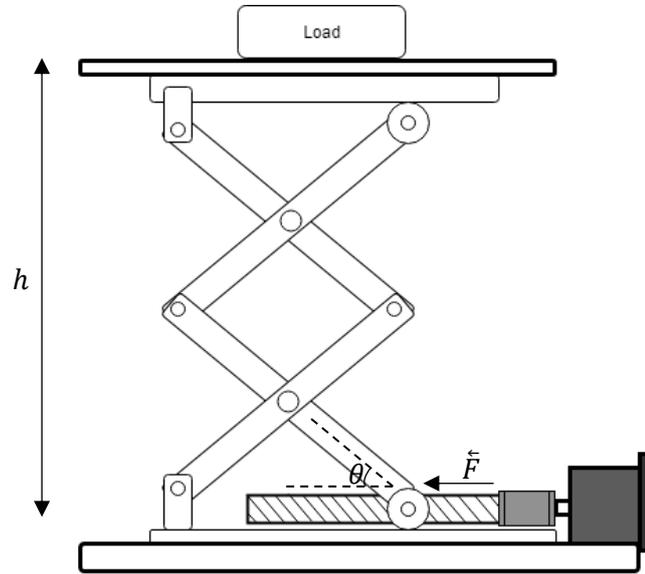
Figure 4.4: Scheme of scissor mechanism with screw jack and stepper motor.
