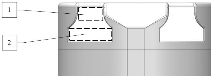
Figure 3.9: Profile of the holes for grabbers. 1 – Upper, smaller part of the hole for the forks; 2 – lower, bigger part of the hole.
