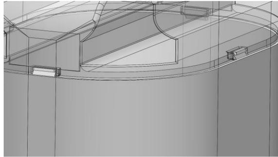
Figure 3.8: Latches for keeping the box closed.
