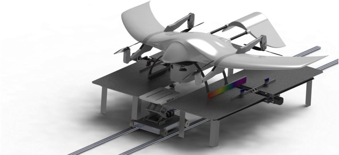
Figure 5.8: Full assembly of the drone delivery system.
