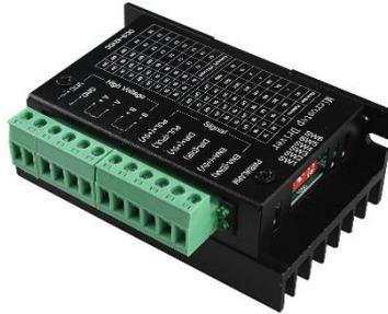
Figure 0.1: TB6600 Stepper motor driver [22].
