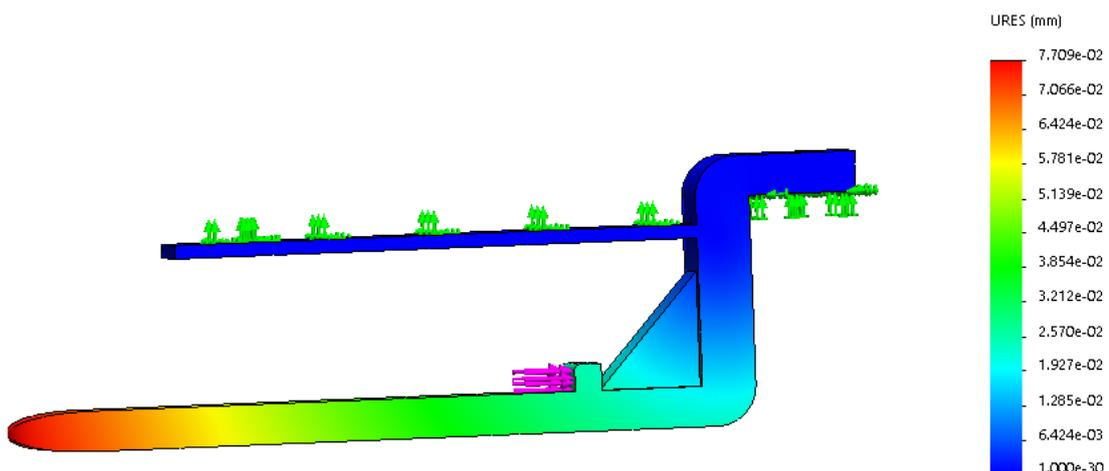
Figure 6.3: Displacement under horizontal force of 10 N is 0.08 mm.
