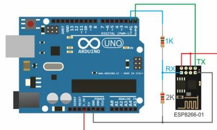
Figure 0.7: Example of connection of Arduino Uno and ESP8266 with resistors [40].
