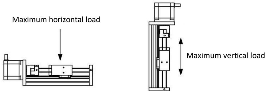
Figure 3.5: Scheme of loads direction. Since the module is performing pushing function, maximum vertical load is important for the project [21].
