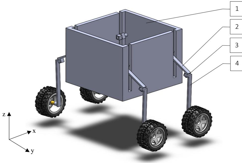
Figure 2.5: Concept of smart courier design. 1 – Box for a payload; 2 – upper part of the leg; 3 – knee; 4 – lower part of the leg with wheel.
