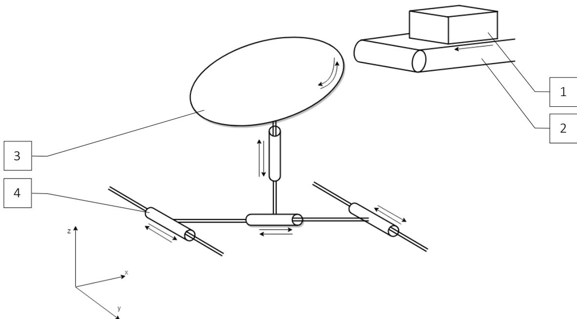
Figure 2.1: Scheme of suggested delivery system with a conveyor (on the right) and a 3-axis platform (in centre). 1 – Cargo box; 2 – Conveyor between a user and the drone; 3 – landing platform for drone; 4 – motors installed on shafts.
