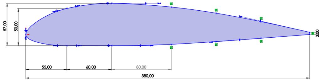
Figure 5.4: One of the sketches for the wing.
