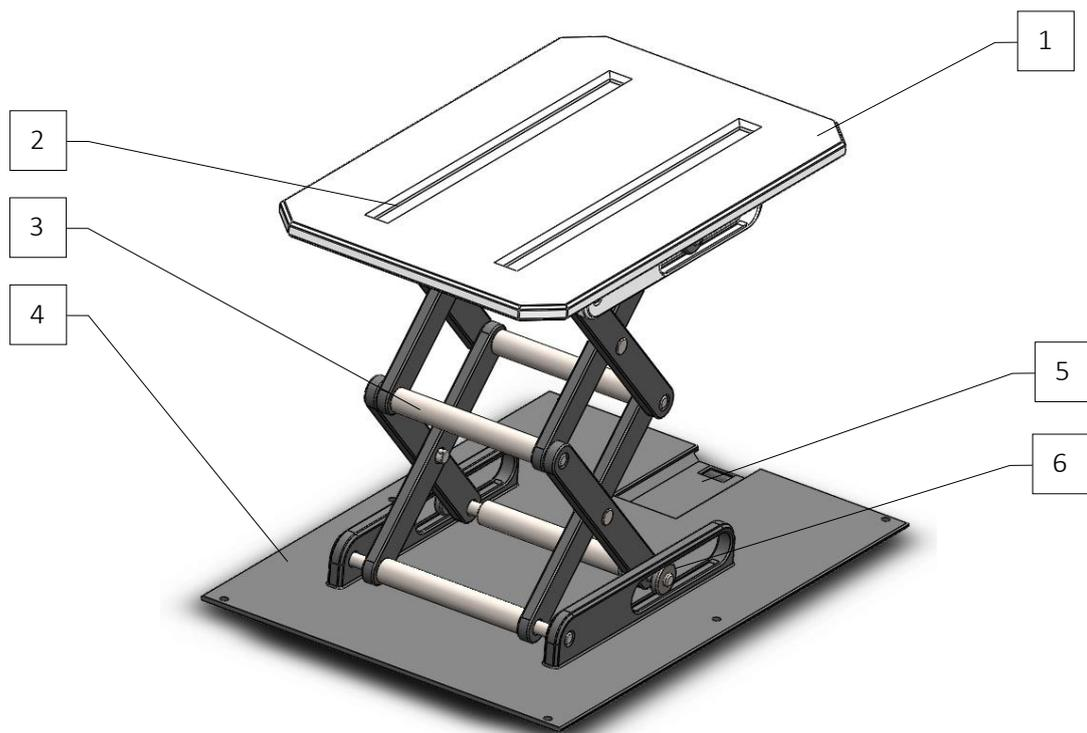
Figure 4.5: Created model of scissor mechanism. 1 – top platform for cargo box; 2 – sockets for the “legs” of the cargo box; 3 – support; 4 – base of scissor lift; 5 – socket for stepper motor; 6 – wheel for the support with buttress thread.
