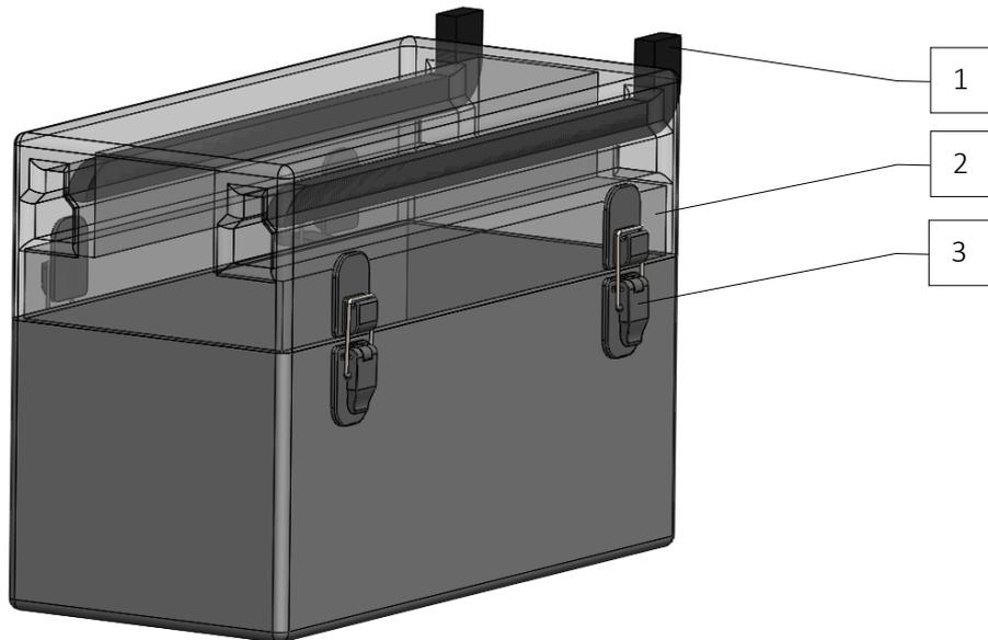
Figure 2.9: Cargo box with fork type grabber. 1 – Fork type grabber, the upper part of it is attached to the bottom of drone; 2 – top of the cargo box with two necessary holes for the fork; 3 – latches to keep the cargo box closed during the delivery process.
