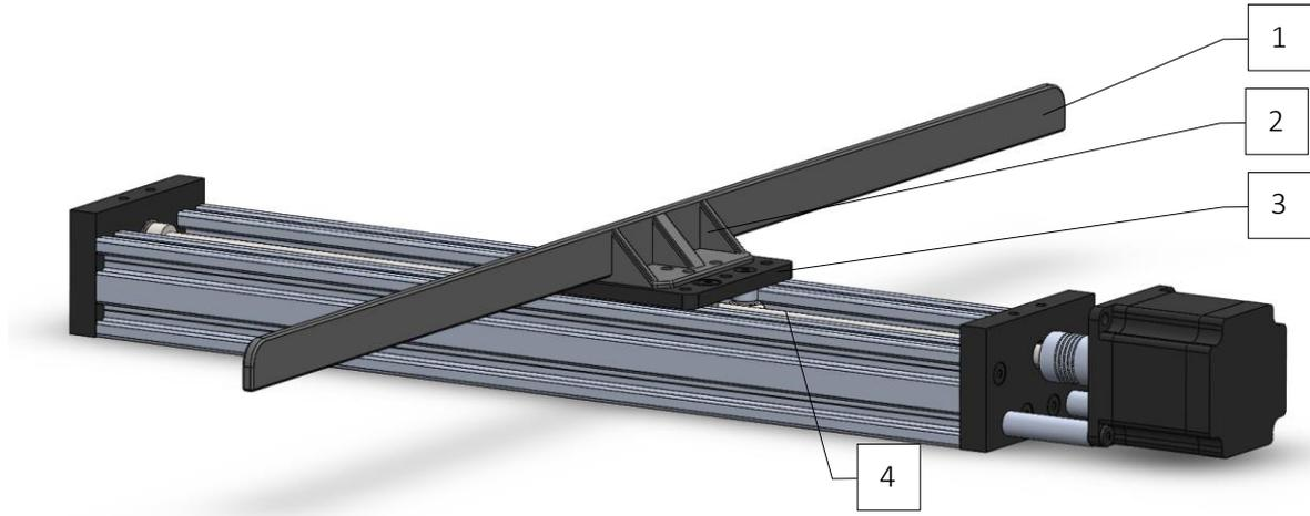
Figure 3.2: Modified linear rail guide (C-Beam linear actuator). 1 – Pusher with 2 – ribs; 3 – platform; 4 – shaft [13].
