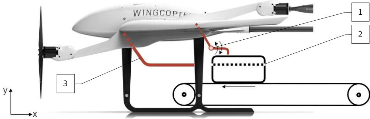
Figure 2.7: Sketch of fork type grabber on the Wingcopter's photo. Fork and anchorage are in red. 1 – Anchorage with servomotor; 2 – cargo box with a hole for the fork coming on a conveyor; 3 – the grabbing fork.
