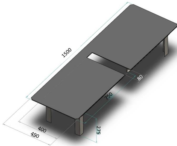
Figure 3.1: Landing platform sizes. All the dimensions are in millimetres.
