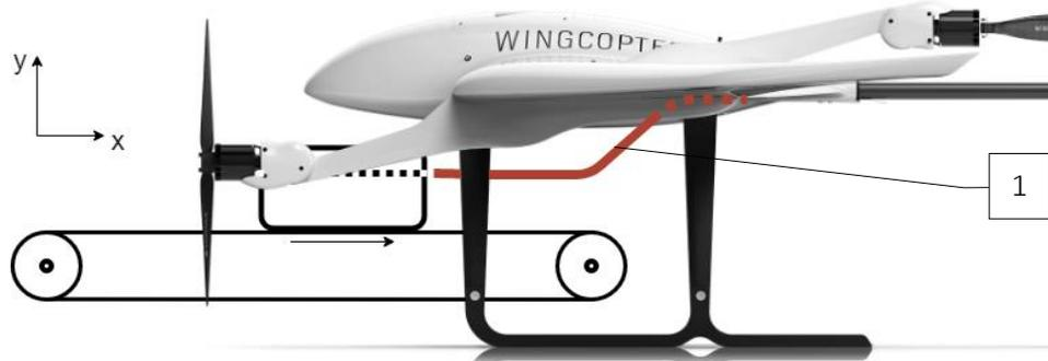
Figure 2.8: Modified sketch of fork type grabber (red). Now it is directed to the head of the drone. 1 – Grabbing fork is installed closer to the end of the fuselage.
