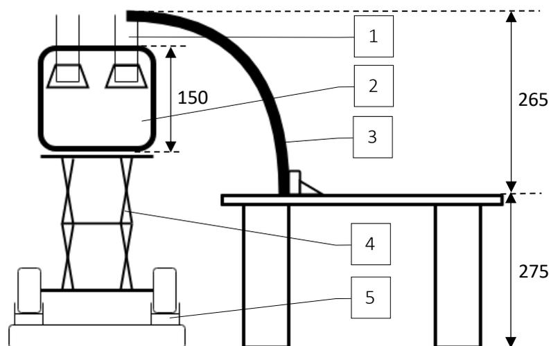
Figure 4.3: Sizes on scheme of delivery system. 1 – Drone’s grabbers; 2 – Cargo box; 3 – Legs of drone; 4 – elevator trolley with scissor mechanism; 5 – rails for the trolley. Dimensions are given in millimeters.
