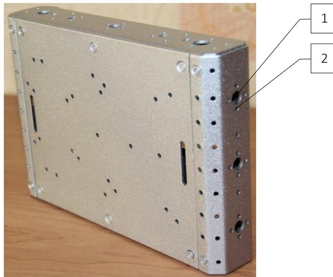
Figure 4.6: Universal chassis for the robots. 1 – Hole for a shaft of the DC motor, 2 – holes for fixing the motor [29].
