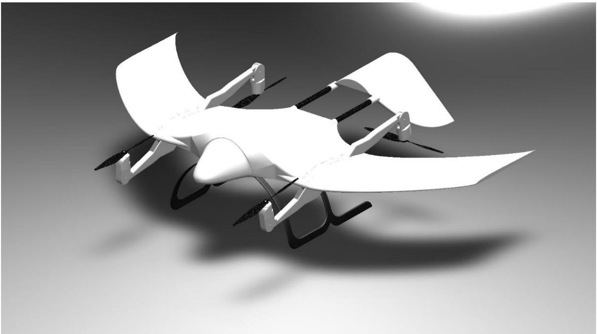
Figure 5.3: Final model of the drone in SolidWorks.
