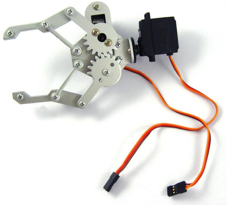
Figure 2.6: Robotic claw with servomotor [15].
