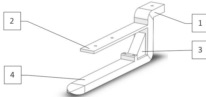
Figure 3.6: One of two branches of grabbing fork for the drone. 1 – Fixing part on the bottom of drone at back side; 2 – fixing part under the bottom of drone at front side; 3 – rib; 4 – place where the cargo box will be carried on.
