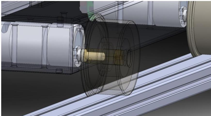
Figure 4.9: Wheel and profile matching.
