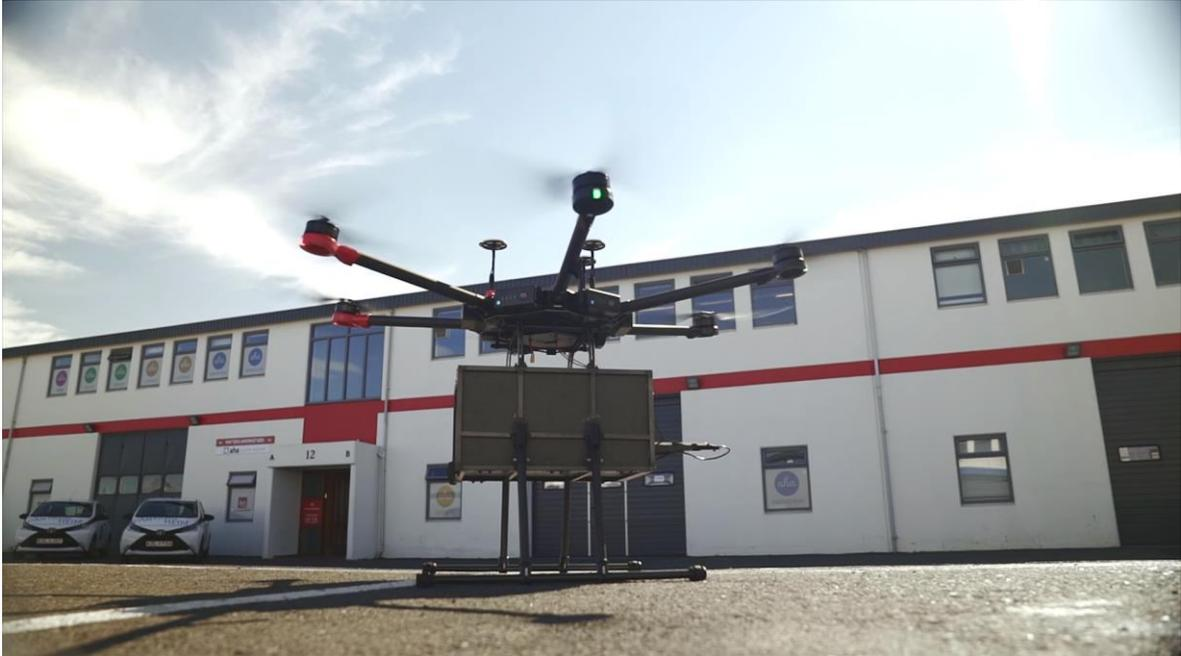
Figure 1.2: Modified DJI Matrice 600 is the main vehicle of Flytrex for deliveries [4].
