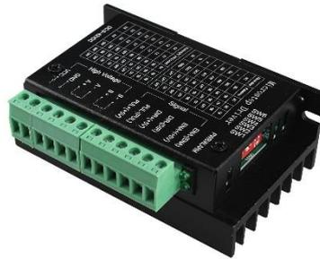
Figure 0.1: TB6600 Stepper motor driver [22].
