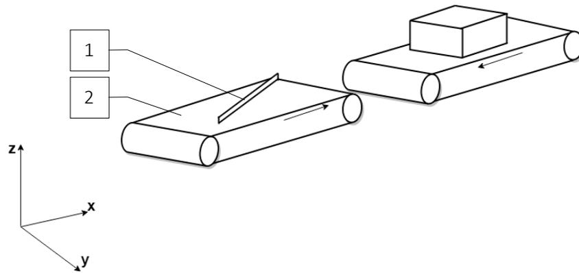
Figure 2.2: Scheme of delivery system with position adjusting conveyor. 1 – An obstacle installed on the conveyor in certain degree; 2 – conveyor as a landing platform.
