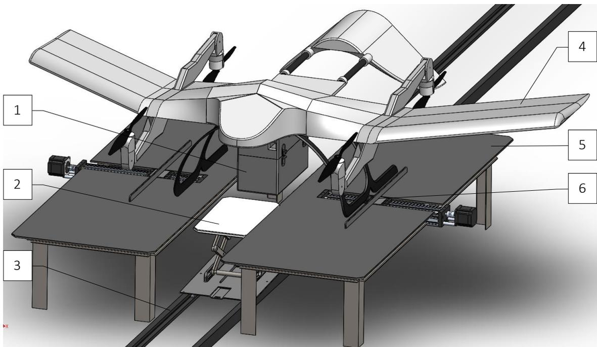
Figure 2.12: Rough model of the delivery design. 1 – Cargo box; 2 – courier-elevator; 3 – rails for courier-elevator; 4 – Wingcopter 178; 5 – landing platform; 6 – pushing mechanism.
