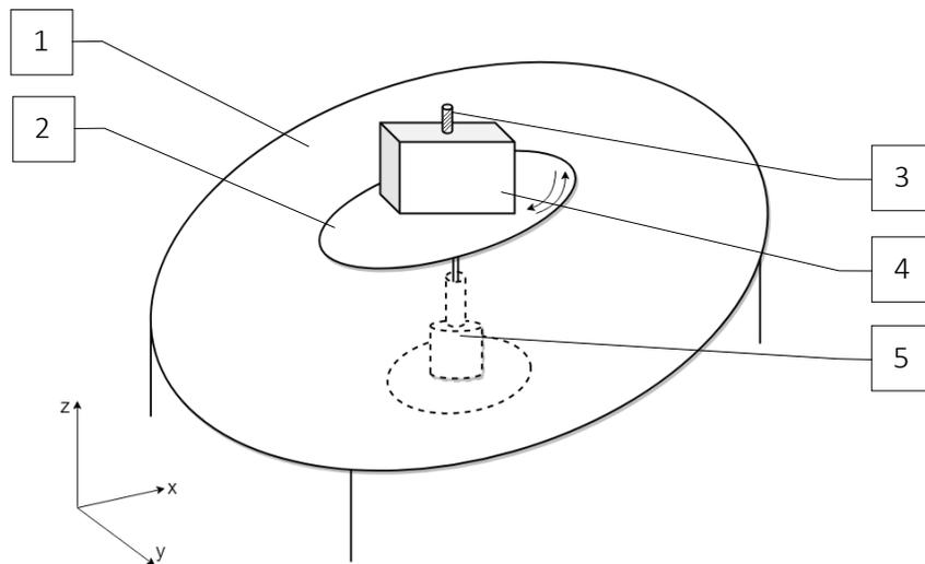
Figure 2.4: Scheme of delivery system with rotating platform. 1 – Big static landing platform; 2 – smaller rotating platform for cargo box; 3 – screw for attaching the cargo box to the drone; 4 – cargo box; 5 – base of smaller platform with motor, shaft etc. which will be under the landing platform.
