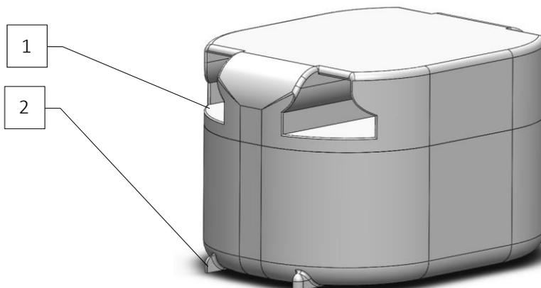
Figure 3.7: Model of the cargo box. 1 – Hole for grabber; 2 – “legs” of cargo box.
