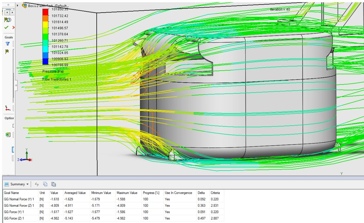
Figure 6.2: Air flow simulation results. Additional force on Z-axis is around 5 N.
