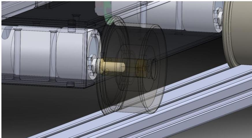
Figure 4.9: Wheel and profile matching.
