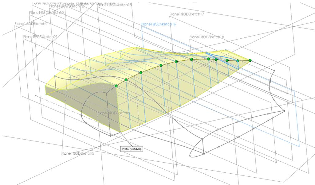
Figure 5.6: Loft operation for half of the body of the drone.
