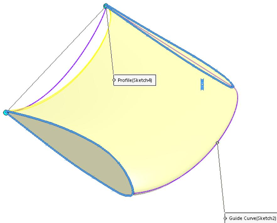
Figure 5.5: Loft operation. You can see how yellow line (automatically created by Loft operation) does not match with violet line (sketch line) at the back side of the wing.
