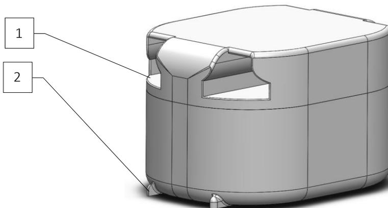
Figure 3.7: Model of the cargo box. 1 – Hole for grabber; 2 – “legs” of cargo box.
