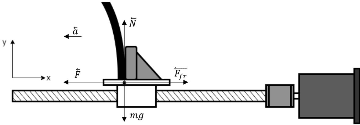
Figure 3.3: Schematic illustration of pushing mechanism during the work process.
