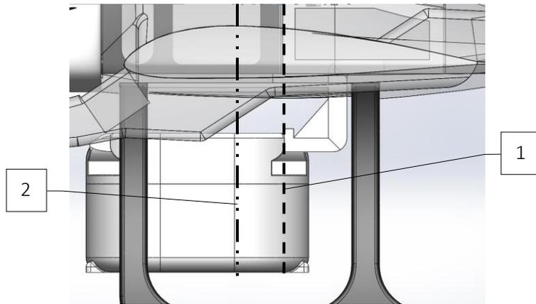
Figure 3.10: Fork and cargo box under the drone. 1 – Original centre of mass of the drone; 2 – new centre of mass of the drone with the same position of batteries.
