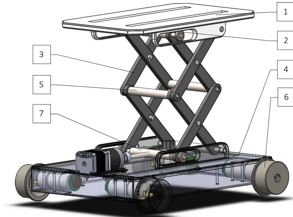
Figure 4.1: Final model of scissor lift created on chosen components. 1 – Top platform; 2 – supporting wheel; 3 – arm; 4 – base (chassis); 5 – support; 6 – main wheel; 7 – support with buttress thread.
