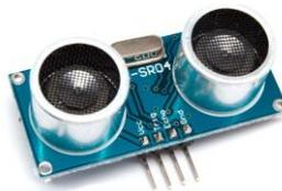
Figure 0.8: HC-SR04 ultrasonic sensor [41].
