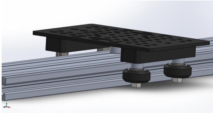
Figure 2.3: Model of V-slot belt driven actuator [13] as an example of landing platform instead of using a conveyor.
