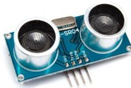
Figure 0.8: HC-SR04 ultrasonic sensor [41].
