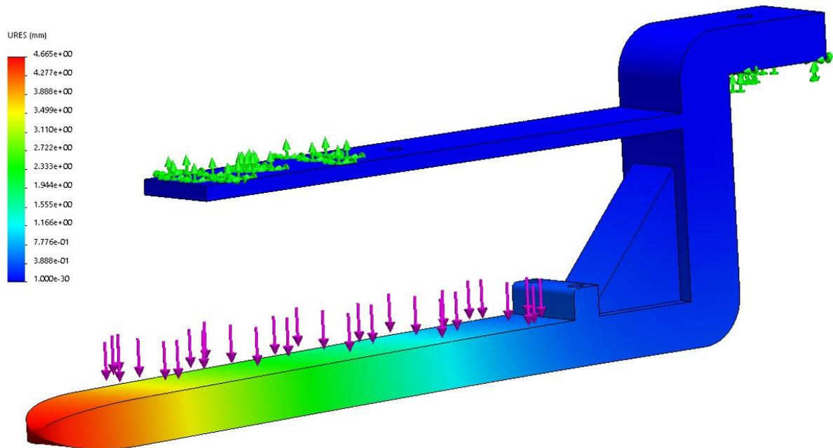
Figure 6.1: Vertical load simulation. Force equals to 40 N. Displacement is 4 mm.
