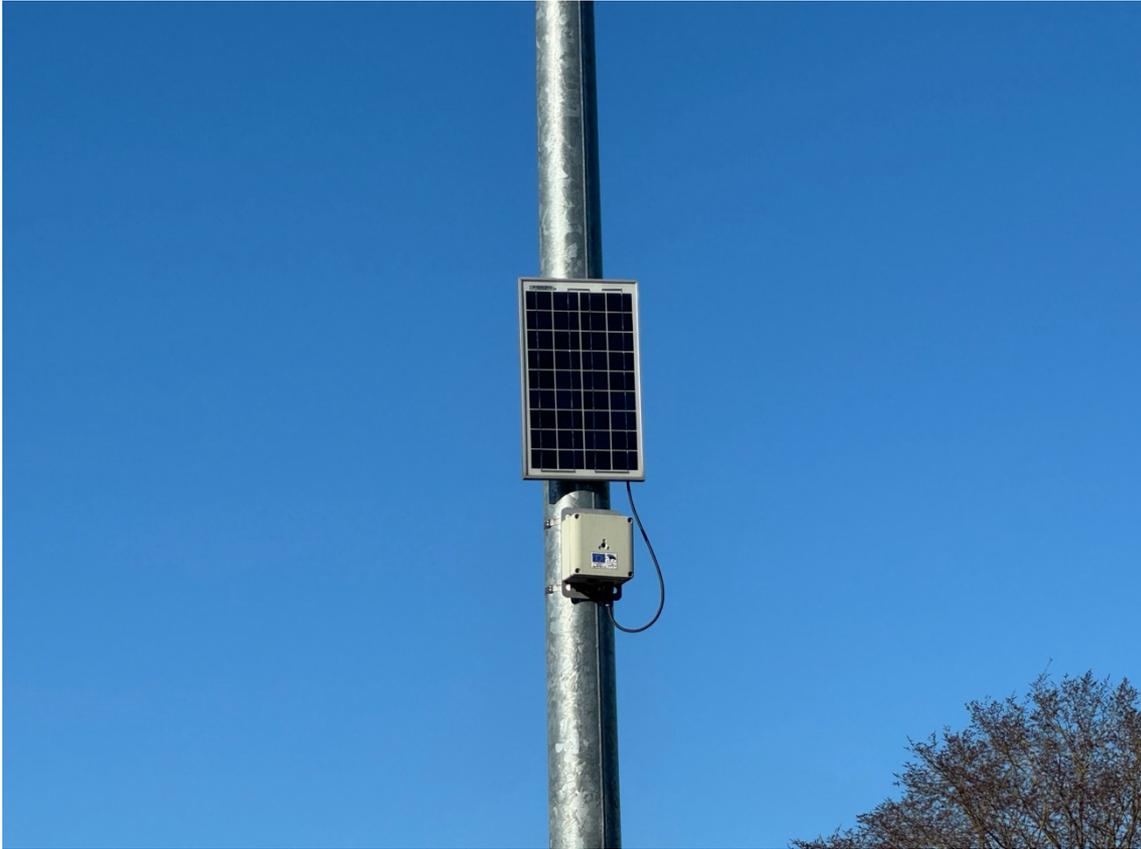
Figure 5. A single microphone SPL sensor installed on a streetlight pole. The device includes a solar panel for energy harvesting and a SPL sensor to monitor urban noise.
