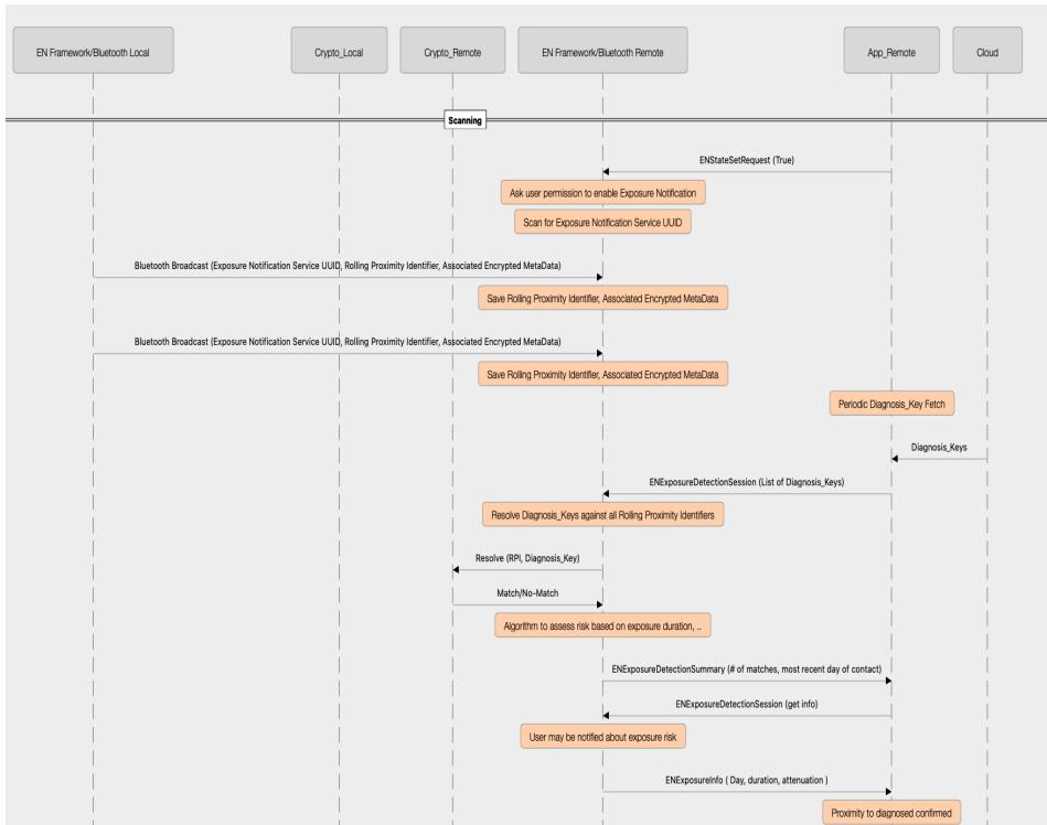
Figure 10. Scanning flow [43].
