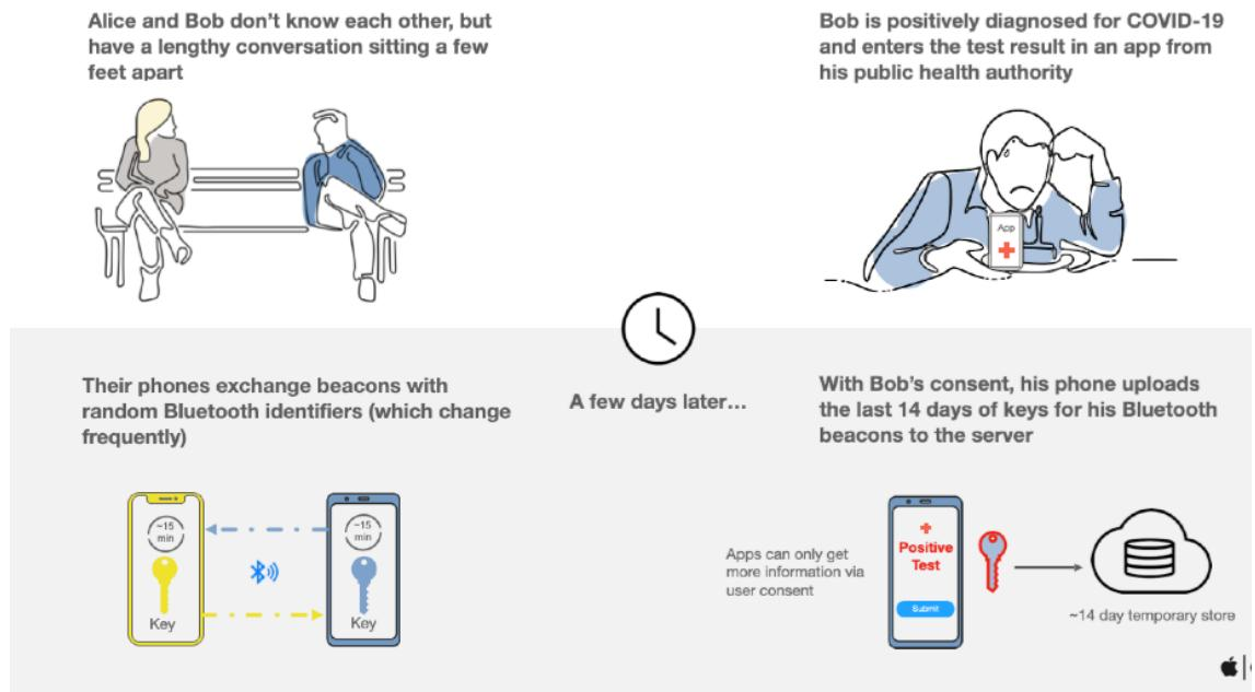
Figure 7. Registering contacts in the GAEN API [42].
