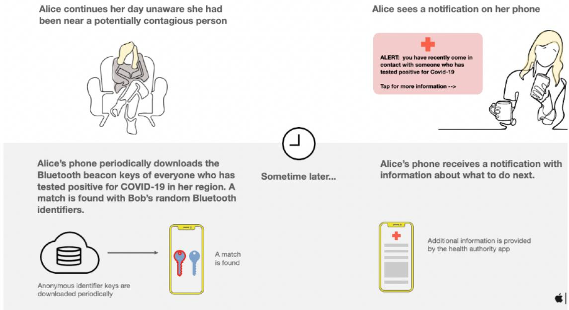
Figure 8. Exposure notification in the GAEN API [42].
