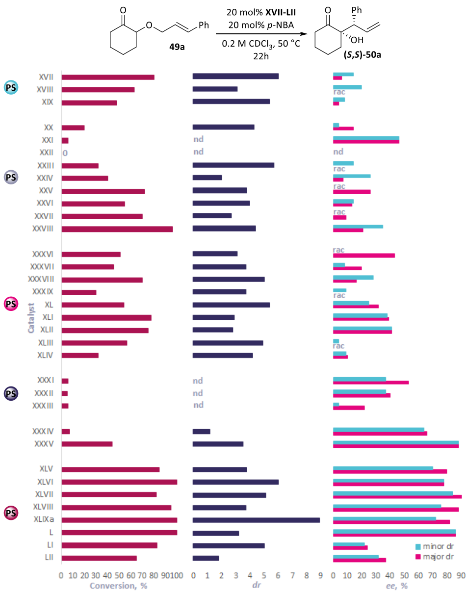
Scheme 39 Screening of immobilised catalysts in the [2,3]-Wittig rearrangement reaction of cyclohexanone derivatives 49a; the diastereoselectivity represents a ratio of X:1
