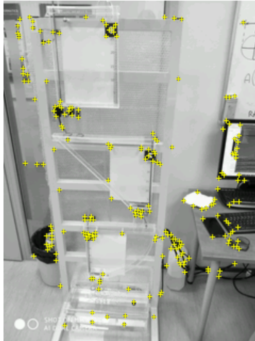
Figure 30. The Vuforia Engine Recognition of Smartphone camera picture
