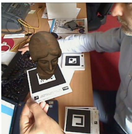
Figure 2. Marker-based AR used to overlay a model on a marker
