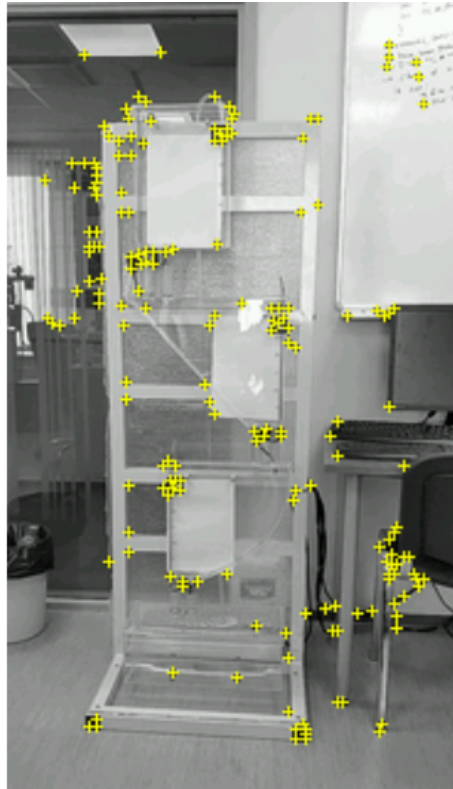
Figure 31. The Vuforia Engine Recognition of AR Camera picture
