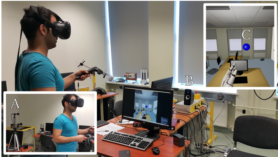
Figure 2.3: Experimental real-time prototype setup. Elements on image: A—Microphone array; B—Emulated sound source (Bluetooth speaker); C—Spherical visualization as it appears in the recreated room VR environment
