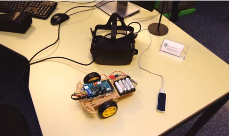
Fig. 10. The physical vehicle joined with leap motion and arduino
