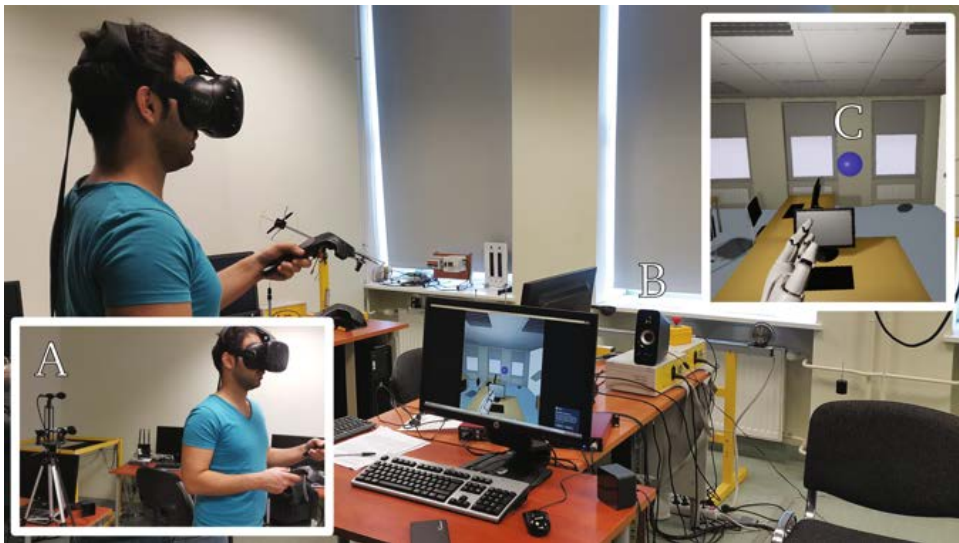
Fig. 5. Experimental real-time prototype setup. Elements on image: A—Microphone array; B—Emulated sound source (Bluetooth speaker); C—Spherical visualization as it appears in the recreated room VR environment
