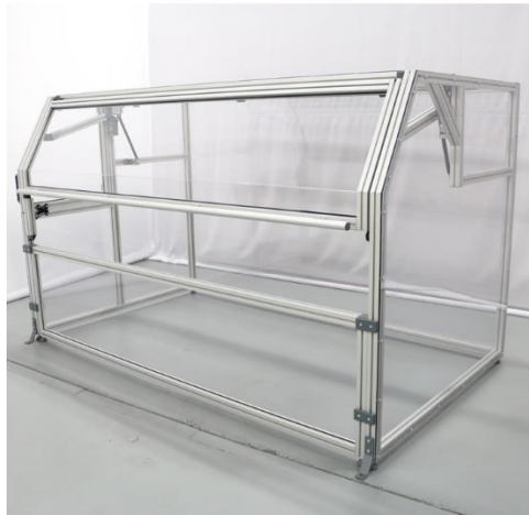
Figure 5.7 Double hinged fold open door in closed position [5]
