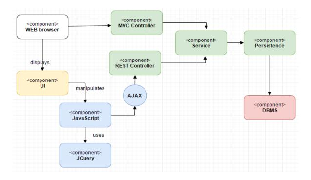
Figure 26 Application Components and their interactions.
