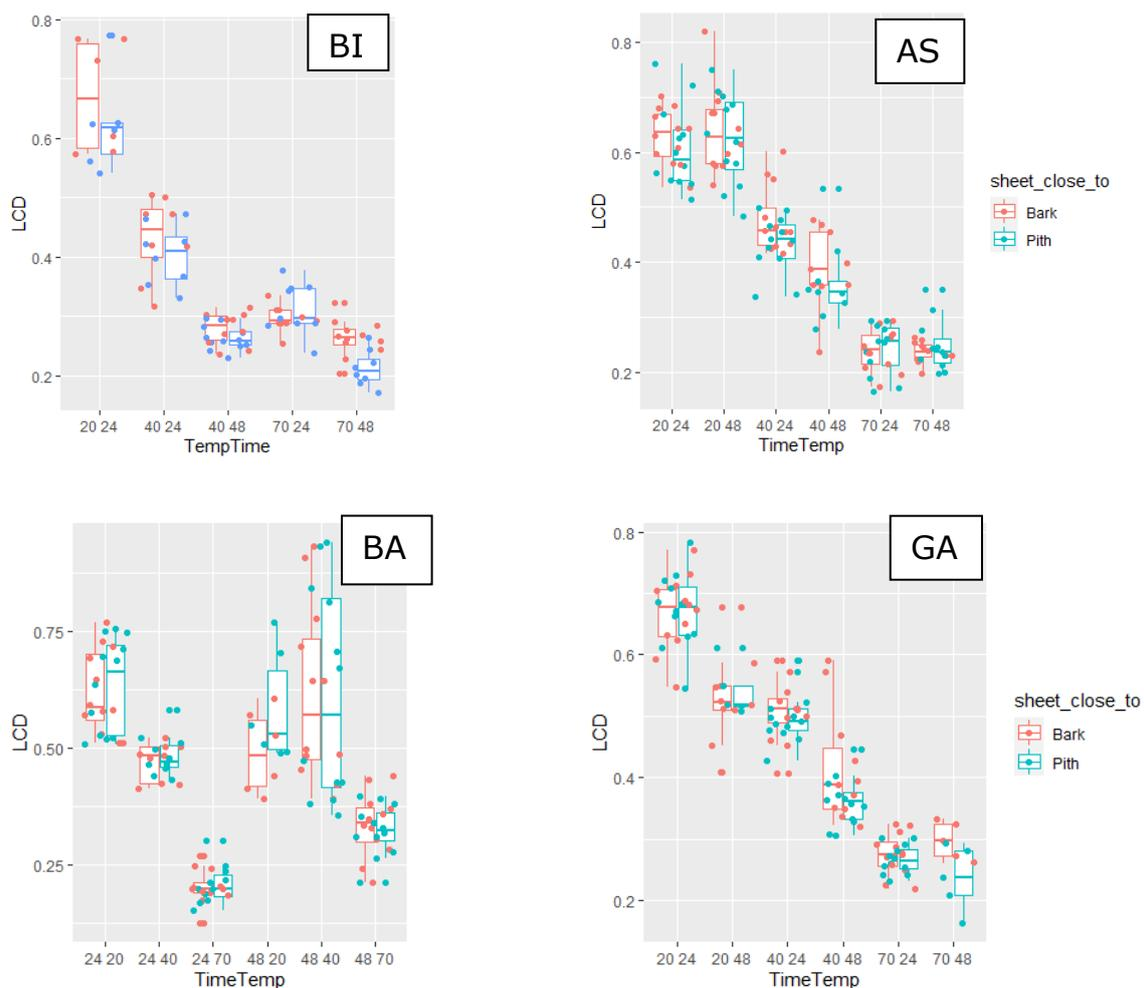
Figure 3.11. Boxplot indicating the variation of lathe checks depth (LCD) between veneer sheets close to the bark and pith at different soak temperatures and soak time.
