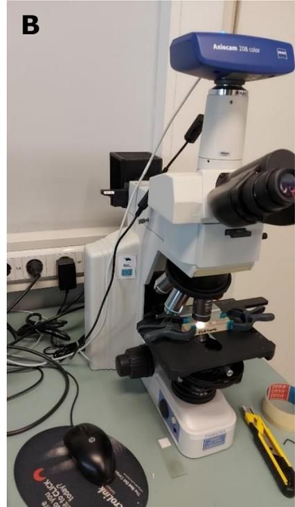
Figure 2.8. A – Dino-lite digital microscope setup, B – Nikon Eclipse microscope.
