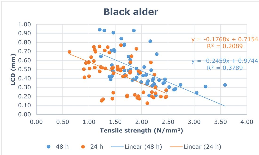
Figure 3.14. Scatter plot showing relationship LCD and tensile strength of black alder soaked for 24 and 48 h.
