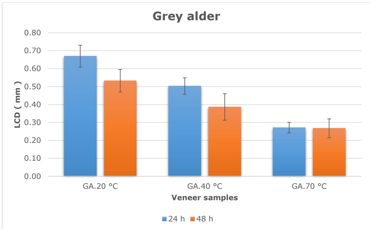
Figure 3.10. Average lathe checks depth (LCD) at different soak temperatures and soak time for grey alder species.
