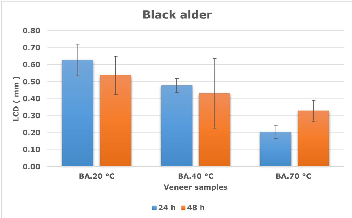
Figure 3.9. Average lathe checks depth (LCD) at different soak temperatures and soak time for black alder species.
