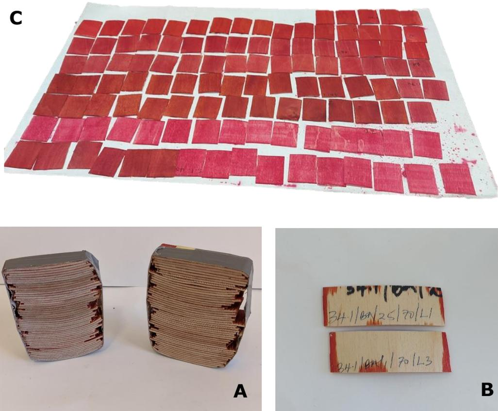
Figure 2.7. A, B - Dyed veneer specimen cut to 20 x 50 mm, C - loose sides stained with Dylon dye
