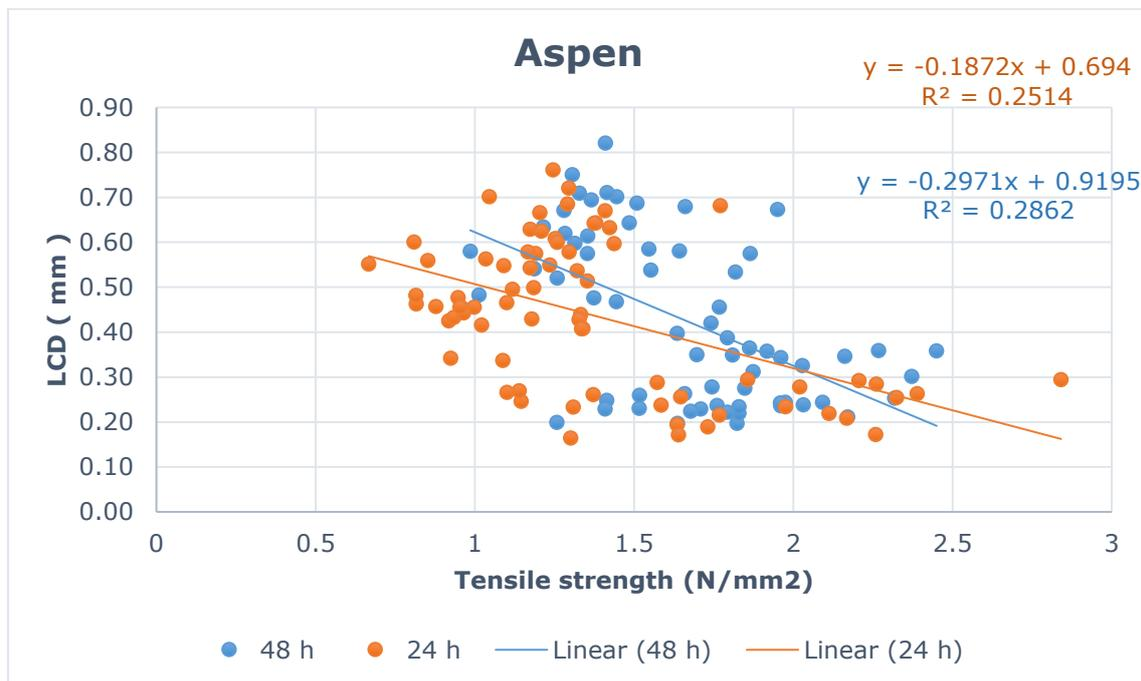
Figure 3.12. Scatter plot showing relationship LCD and tensile strength of aspen soaked for 24 and 48 h.
