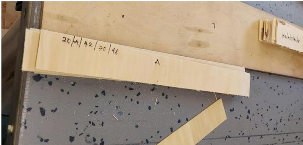
Figure 2.4. Cutting of veneer strips for tensile testing
