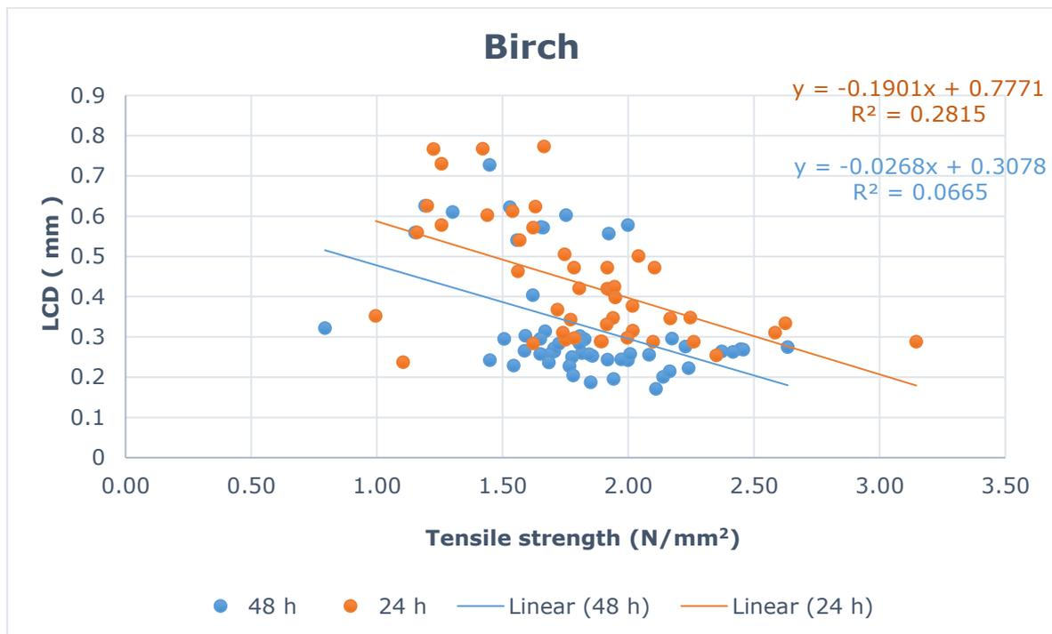
Figure 3.13. Scatter plot showing relationship LCD and tensile strength of birch soaked for 24 and 48 h.
