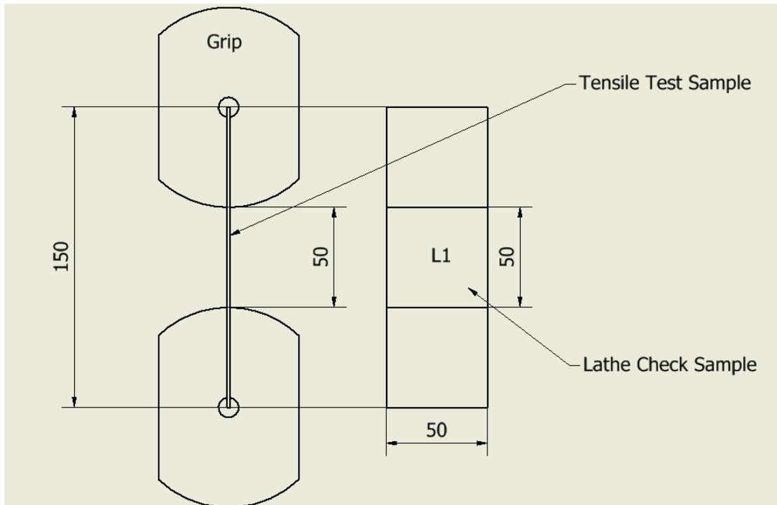
Figure 2.5. Tensile test sample gripped between clamps and equivalent lathe check sample placed alongside
