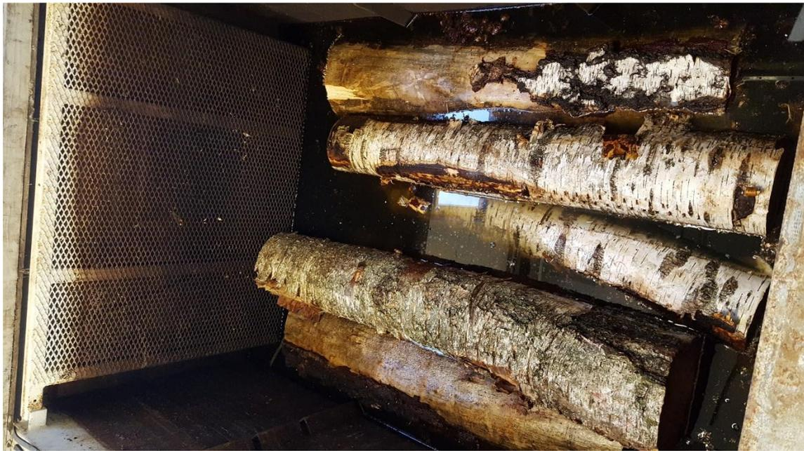
Figure 2.1. Peeler blocks placed in soaking bath
