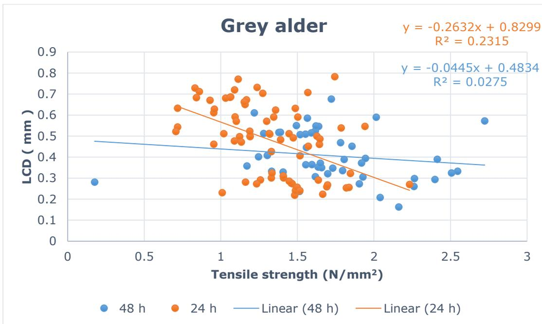
Figure 3.15. Scatter plot showing relationship LCD and tensile strength of grey alder soaked for 24 and 48 h.
