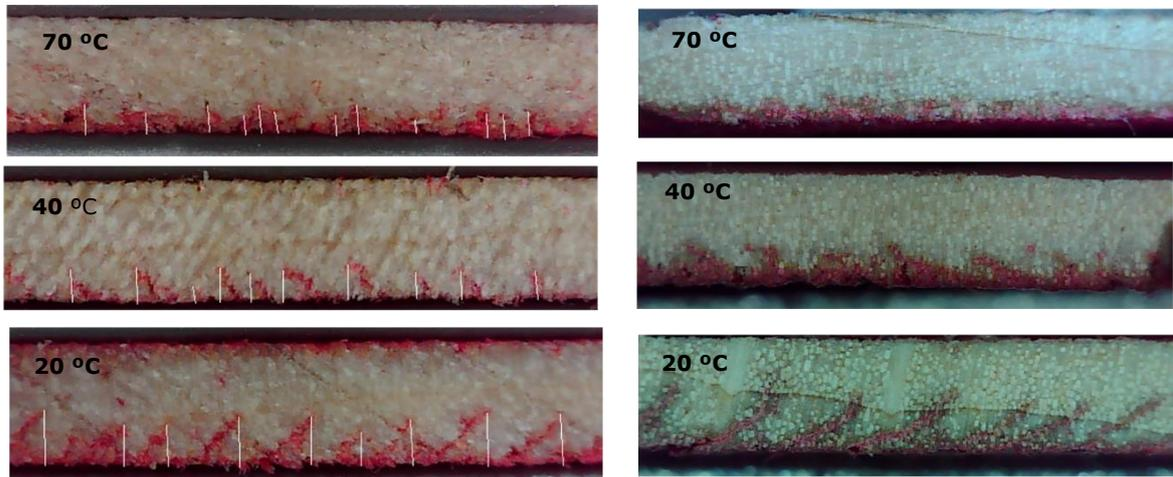
Figure 3.6. Captured images of lathe checks depth at different soak temperatures
