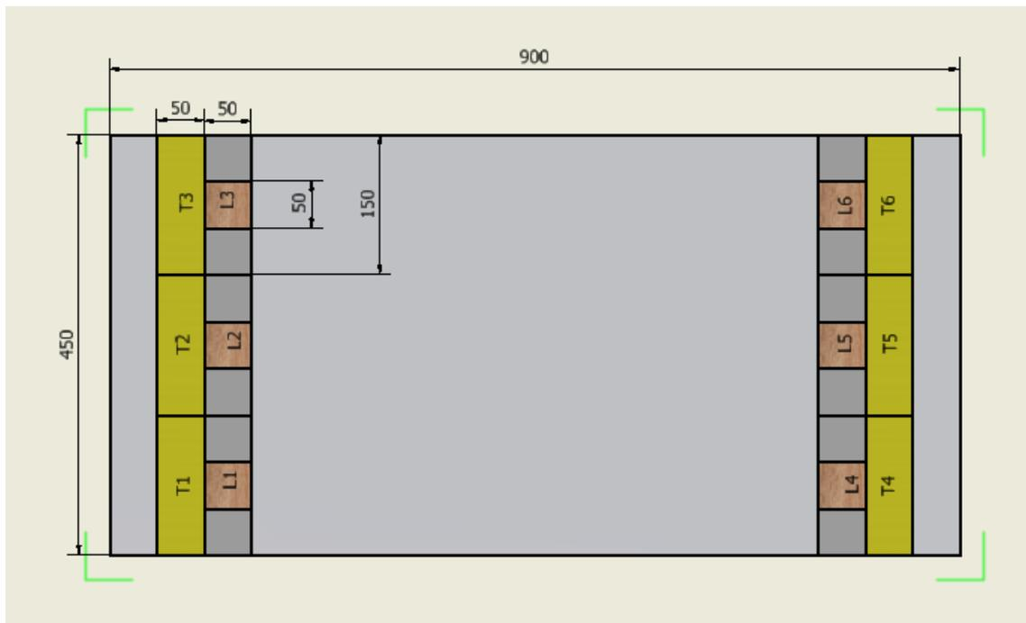
Figure 2.6. Cutting pattern for tensile test and lathe check samples
