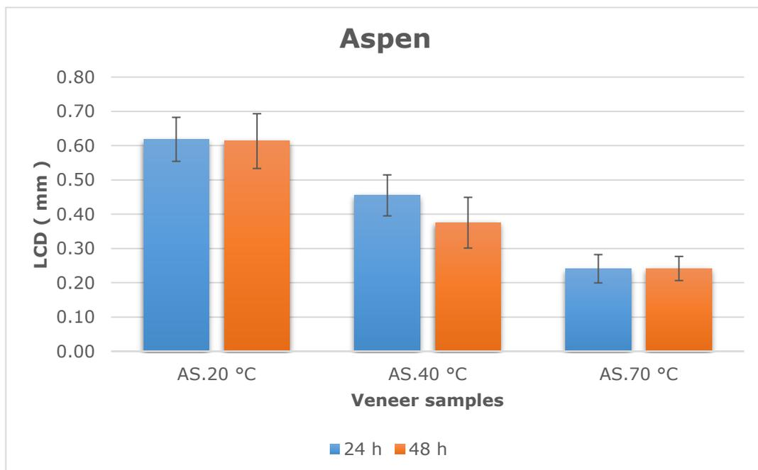
Figure 3.8. Average lathe checks depth (LCD) at different soak temperatures and soak time for aspen species.
