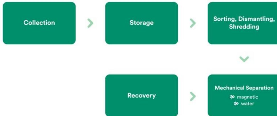
Figure 2.10: The e-waste recycling process flowchart (RTS, 2021)
