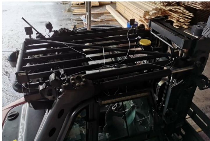
Figure 4.2: Fieldbee GNSS L2 receiver placed on a Forklift
