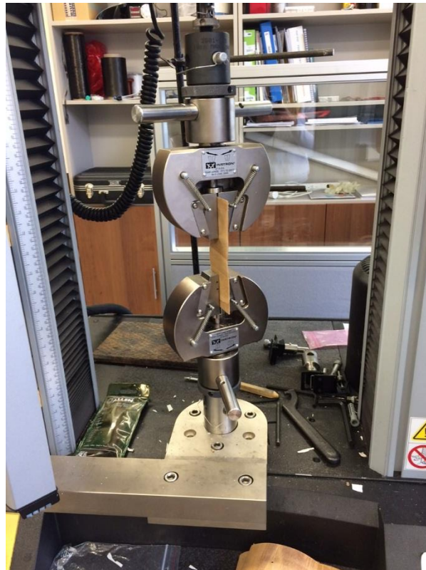
Figure 17. Instron 5866 with false heartwood veneer specimen – (Authors photo 2015)
