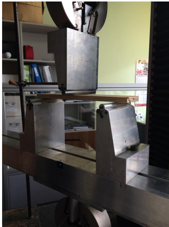
Figure 21. Bending strength in Instron 5866 – (Authors photo)
