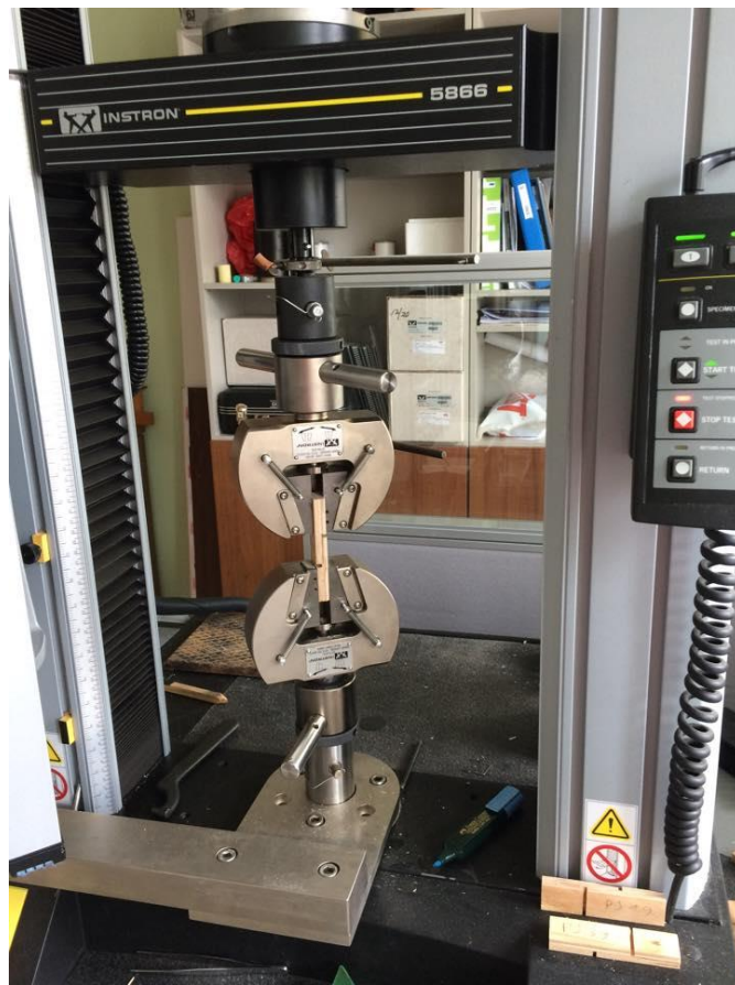
Figure 20. Shear strength testing in Instron 5866 – (Authors photo)
