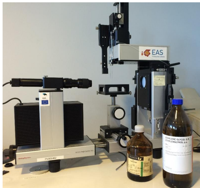
Figure 15. Contact angle system with liquids used in tests – (Authors photo 2015)
