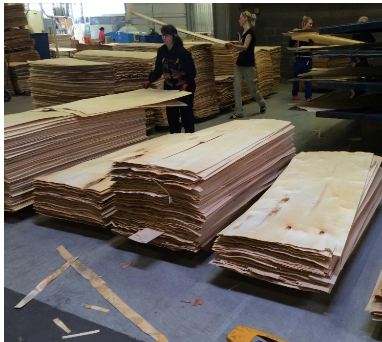
Figure 6. Sorting by classes. From left to right – Class A, BB, BC and C - (Authors photo 2015)
