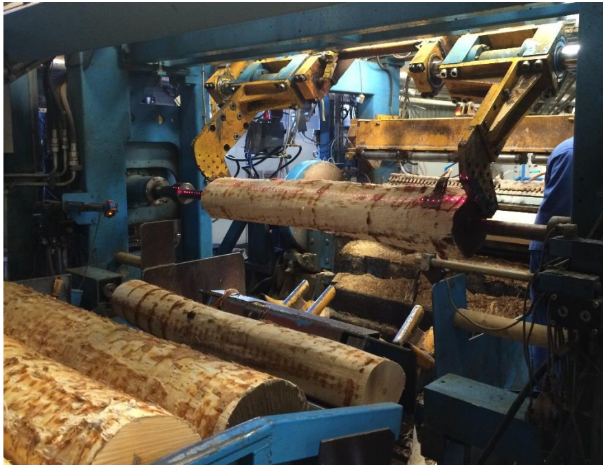
Figure 4. Rotary peeled - (Authors photo 2015)
