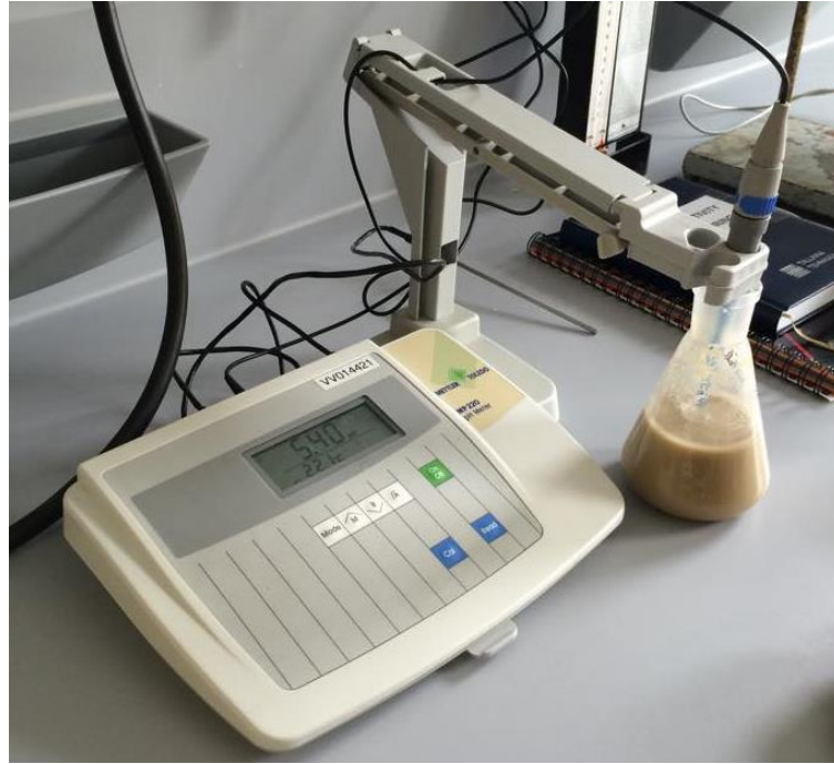
Figure 13. Measuring the pH - (Authors photo 2015)
