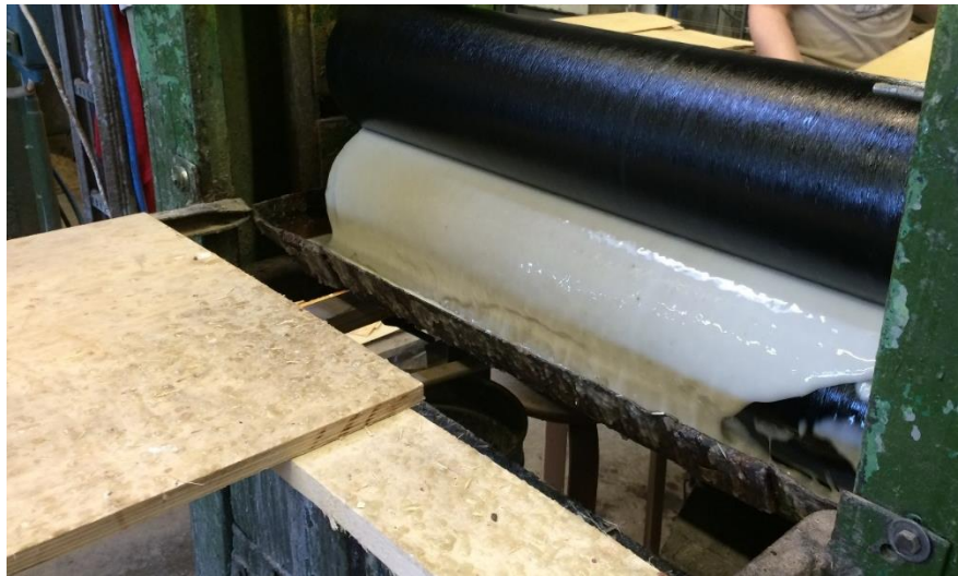
Figure 7. Roller glue spreader - (Authors photo 2015)
