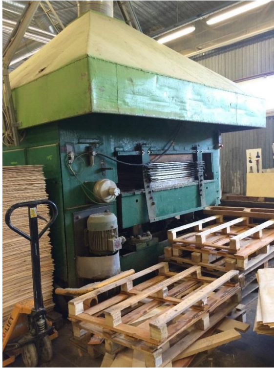
Figure 8. High frequency press - (Authors photo 2015)
