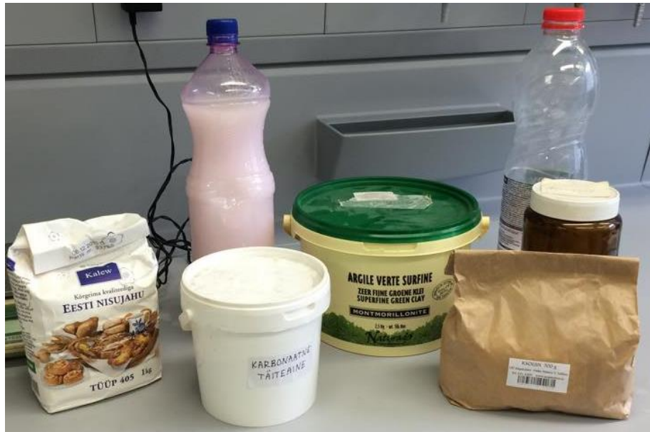
Figure 12. Fillers, from left to right - wheat flour, CaCO 3 , montmorillonite, kaolin, aerosil and UF is in the bottles - (Authors photo 2015)
