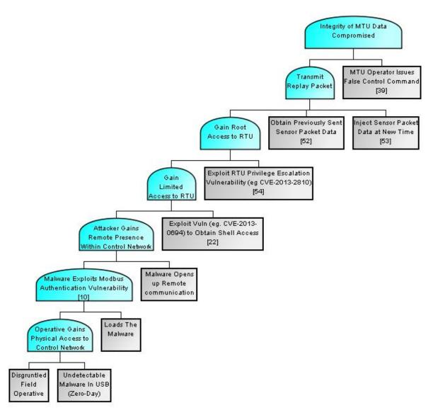
Figure 4. Replay Attack Tree Model
