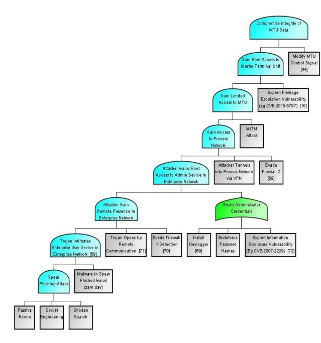
Figure 8. Spear Phishing Attack Tree Model
