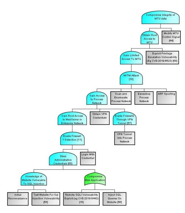
Figure 5. SQL Injection Attack Tree Model
