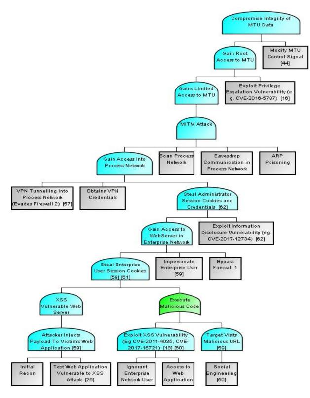
Figure 6. Cross-site Scripting Attack Tree Model
