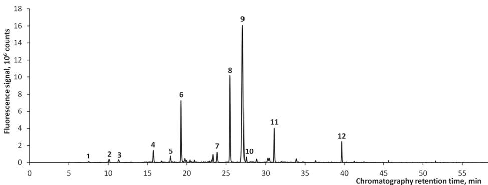
**Figure 1** An example of a HPLC chromatogram of a spent dialysate sample monitored by fluorescence detection at Ex: 280 nm and Em: 360 nm.
