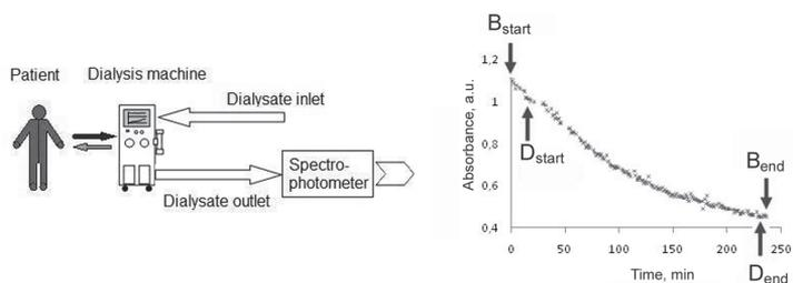
**Fig. 1.** The clinical set-up of the experiments. Time points when the samples were taken for the later analysis are as follows:  $B_{start}$  – blood sample collected before dialysis session,  $B_{end}$  – blood sample collected at the end of hemodialysis,  $D_{start}$  – dialysate sample collected 10 min after the start of hemodialysis,  $D_{end}$  – dialysate sample collected at the end of hemodialysis. The online absorbance measurements after every 30 s are presented by “x”.
