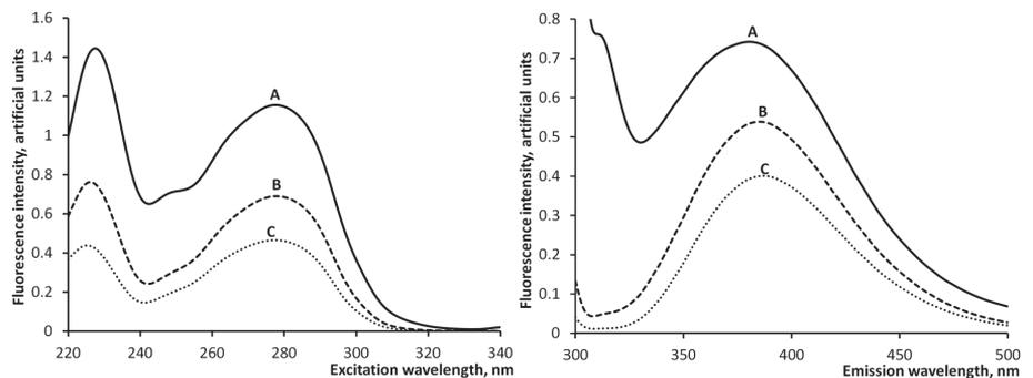
**Fig 5. Comparison of Ex and Em scan spectra between the selected peaks and the whole chromatogram. (A)—total fluorescence, (B)—sum of four identified indoles, (C)—IS.**
