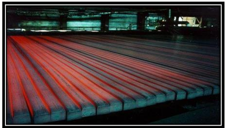
Figure 1. Example of billets(Asg metal ltd)
