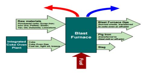
Figure 11. Process scheme of the iron making process. (EMEP/EEA emission inventory guidebook 2009)
