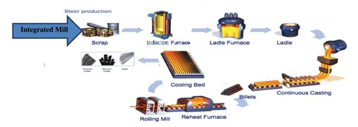
Figure 6: Abbas Steel Manufacturing Process (to be) (Alter Ego 2012)
