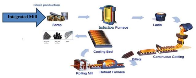
Figure 8: Example of a Abbas Steel Manufacturing Process (As it) (Alter Ego 2012)
