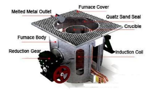
Figure 3. Induction furnace (Weifang Jinhuaxin Electric Furnace Manufacturing)
