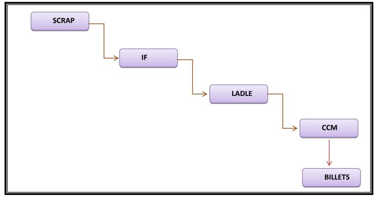
Figure 17. Steel Manufacturing Process Steps
