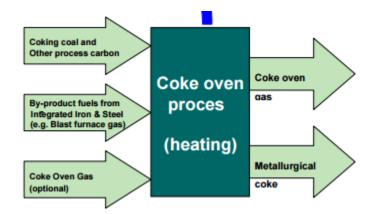
Figure 10. Process scheme of the coke production process. (EMEP/EEA emission inventory guidebook 2009)
