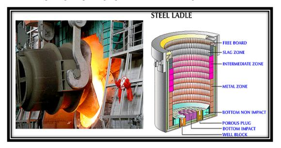
Figure 5. Example of Ladle furnace (kosmokraft Cosmos Power in Refractories)
