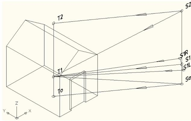
Figure 6. 3D-object (house) with target-points ( $T_0$ ,  $T_1$ ,  $T_2$ ) and camera-points ( $S_0$ ,  $S_1$ ,  $S_2$ ;  $S_{1L}$ ,  $S_{1R}$ ). Even more showy is to create stereogram of 3D-objects. Stereo-effect is based on two-eye seeing. Images for left ( $S_{1L} > T_1$ ) and right ( $S_{1R} > T_1$ ) eye are different (Fig. 7).
