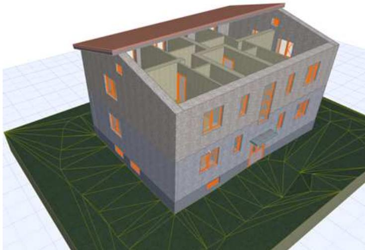
Figure 3. BIM model of building including terrain modelled in ArchiCAD.
