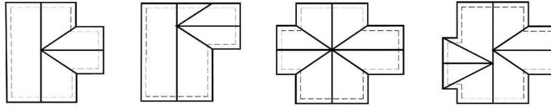
Fig. 3. Principal-type schemes of pitched roof plans
