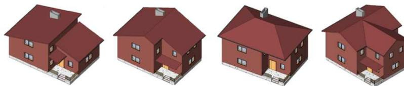
Fig. 1. Roof shapes: mono-pitched, gable and hip roof
