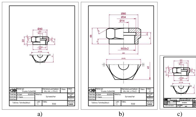
Fig. 1. a) Drawing of the compression nut in scale 1:1 on format A4.
