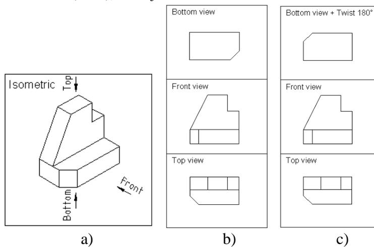
Figure 8. a) source 3D-object; b) 3 views with incorrect Bottom view; c) corrected Bottom view ( $Dview > Twist > 180^\circ$ ). A long-time AutoCAD problem in 3D-modelling is that the Bottom view is rotated  $180^\circ$  (all other views are correct).
