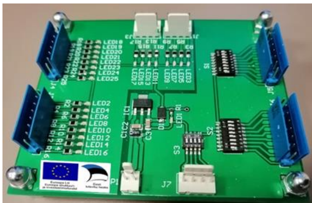
Figure 12. Logic test bench board.
