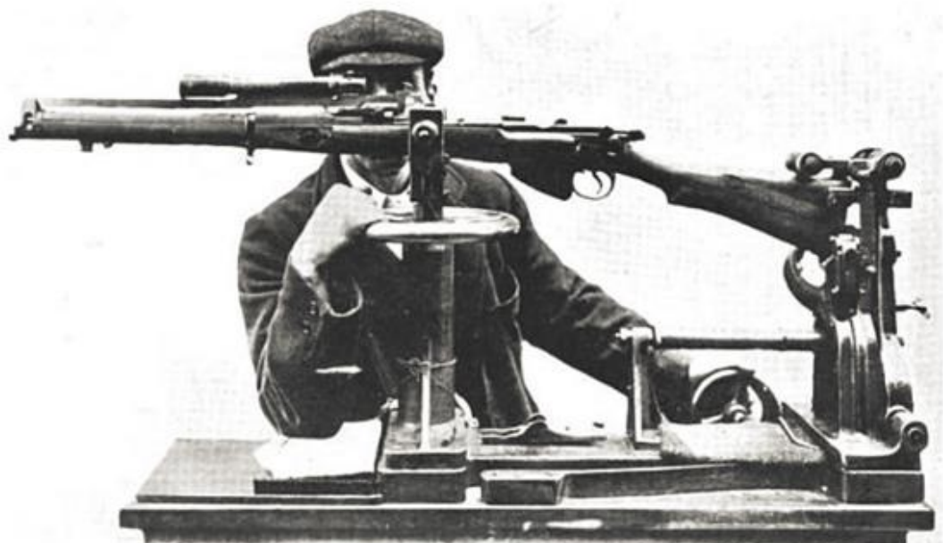
THE MECHANICAL REST USED IN TESTING SERVICE RIFLES
