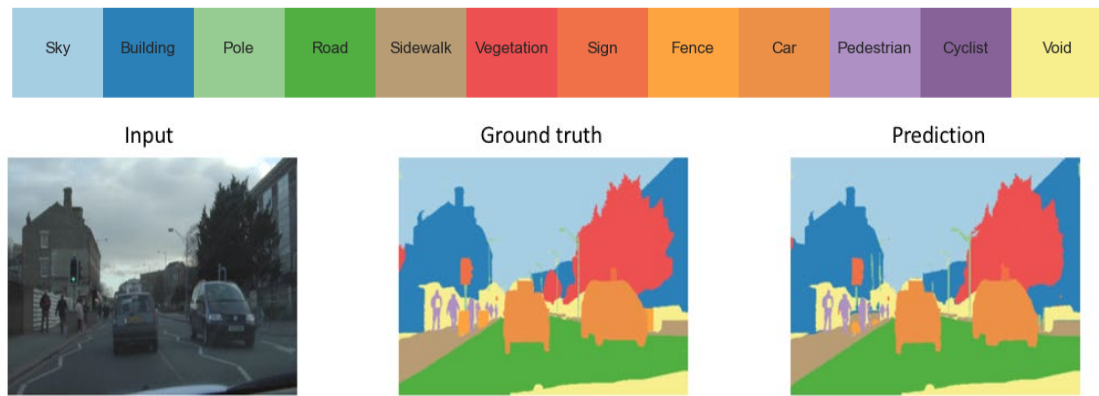
Figure 4: Illustration of Ground Truth Data generation from an input image and the output of from a prediction model. [22]
