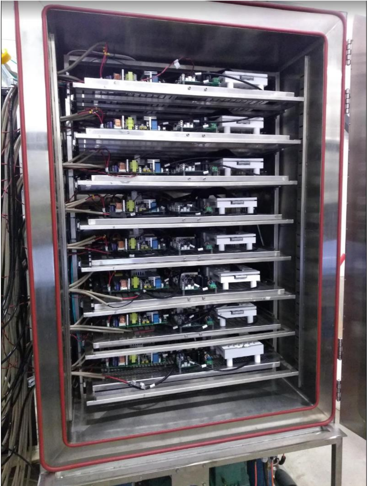
Figure 1.2 Inside view into Arctest climate chamber filled with EUTs
