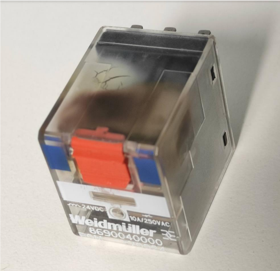
Figure 1.9 Broken fan supply board load relay
