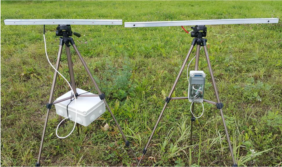
Figure 4.23: Linear array implementations on the BeagleBone Black (left) and on the mote system with Amel microcontroller (right).
