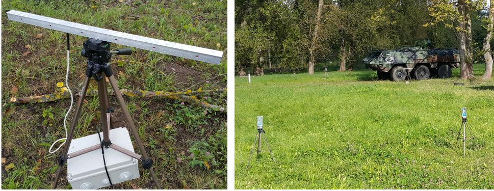
Figure 6.8: Linear array UGS prototype (left) and two data aggregation nodes (right).
