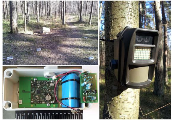
Fig. 2. UGS distribution in real environment (upper left), prototype of acoustic UGS with the microphone amplification circuit (bottom left) and a PIR UGS in a camouflage case designed by Defendec Inc. (right).
