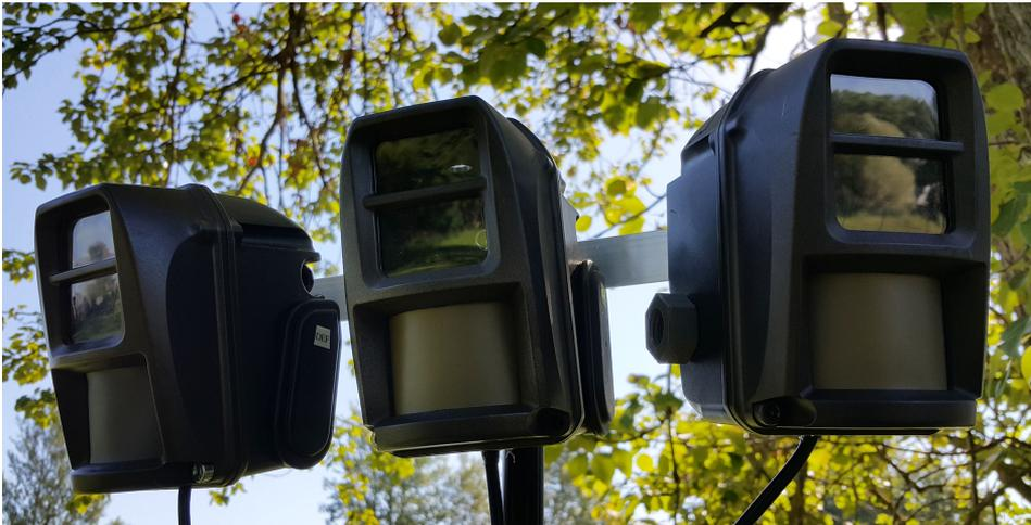
Figure 6.25: PIR sensors encased in a camouflaged chassis designed by Defendec Inc.
