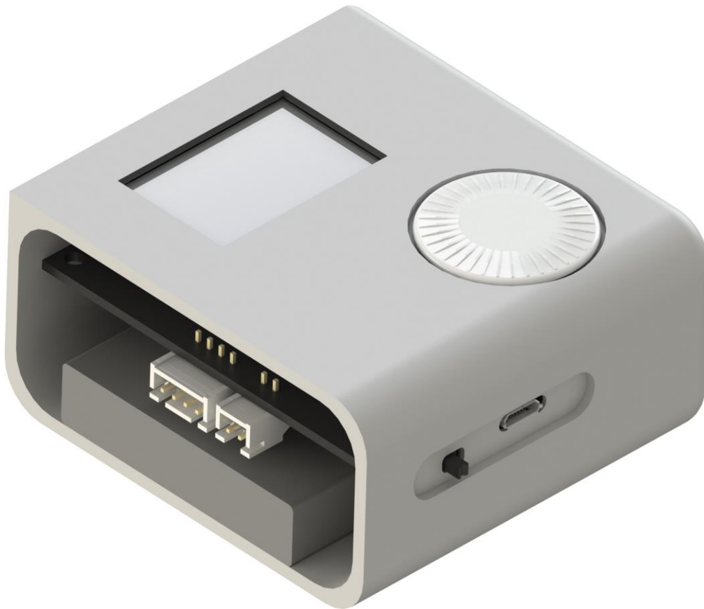
Figure 31. Conceptual model rendering of a section of the enclosure and user interface for the improved electronics design. The grey block under the circuit board represents a Turnigy 4200 mAh LiFePO 4 battery for size reference.
