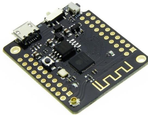
Figure 6. Wemos TTGO MINI32 V2.0 development board[20]
