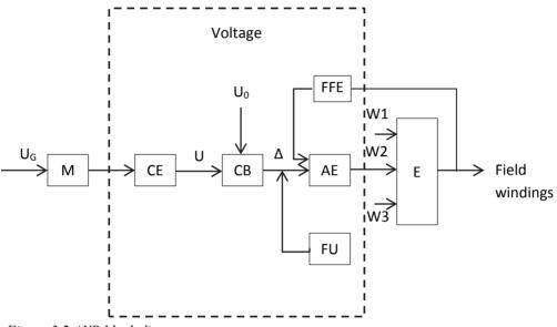
Figure 3.2 AVR block diagram
