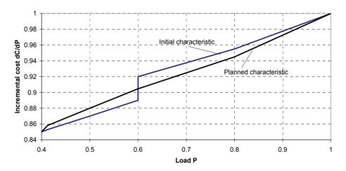
*Figure. 6.3. Initial and planned incremental cost rate characteristics (in relative units) of the power unit.*
