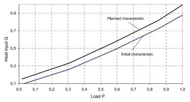
Fig. 2. Initial and planned characteristics of the turbine.
