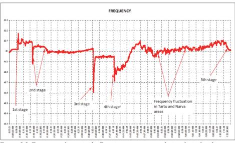
Figure 5.5. Frequency change in the Estonian power system during the isolated operation
