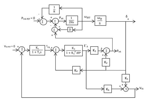
Figure 2.3 Generator block diagram with voltage regulation.
