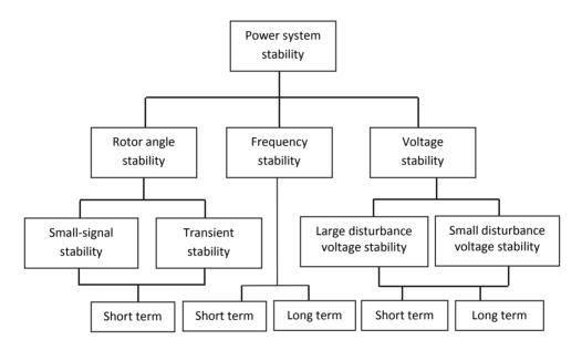
Figure 1.1 Classification of power system stability
