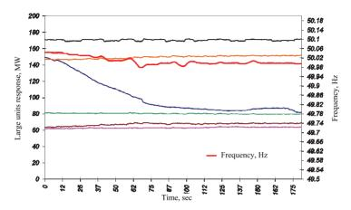
*Fig. 3.* The response of large units to slow changes in generation amount within the isolated system.
