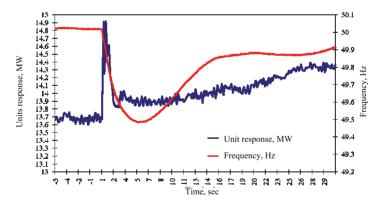
Fig. 4. The small unit response to generation loss event.
