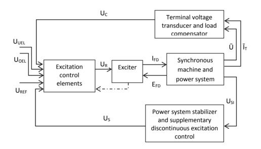
Figure 3.1 General block diagram for a synchronous machine excitation control system
