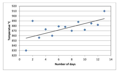
Figure 6.1. Temperature change in the reversing chamber between two boiler cleanings
