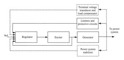
*Fig. 1.* Functional block diagram of the control system of a synchronous generator's excitation.
