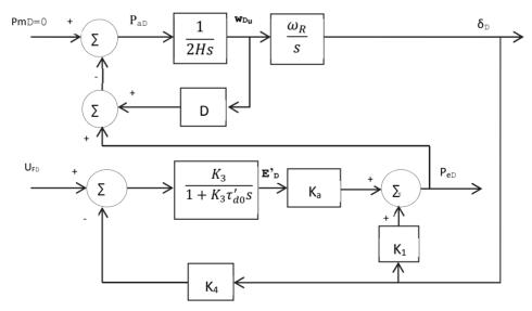
Figure 2.2 Simple linearized block diagram representation of a generator model
