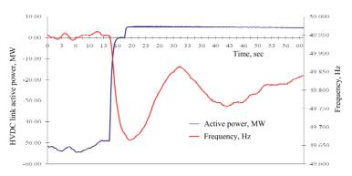
*Fig. 5.* Changes in active power via HVDC link and system frequency in the stage of AFC switch-offs.
