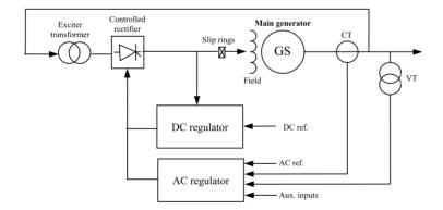
Fig. 2. Scheme of the static excitation system.
