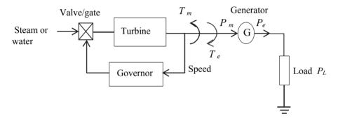
Figure 4.1 Generator supplying isolated load
