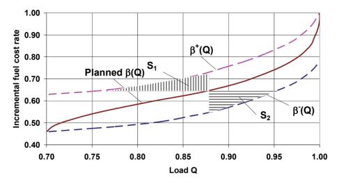
Figure. 6.5. Initial (lower and upper) and planned characteristics of a boiler
