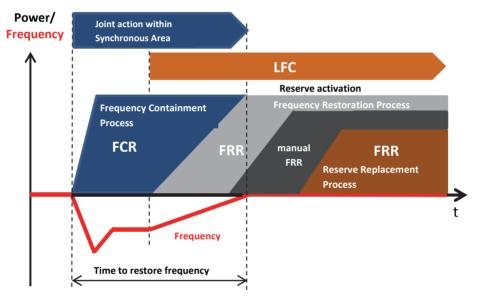
Figure 5.1 shows frequency regulation phases [44].
