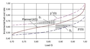
Fig. 4. Initial (lower and upper) and planned characteristics of a boiler.
