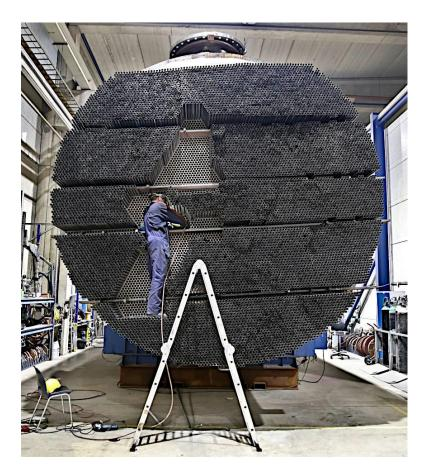
Figure 1.4 Tube heat exchanger in Estanc workshop [3]
