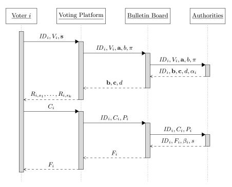
Fig. 3: Sequence diagram of the vote casting and confirmation phase.
