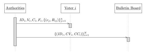
Fig. 2: Sequence diagram of the election preparation phase.
