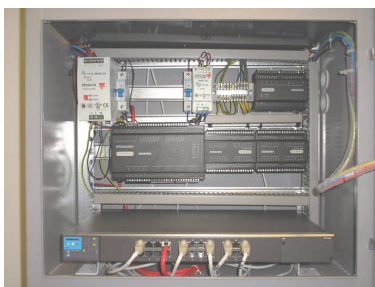
Fig. 6. View of an experimental setup with RTU devices for microgrid experimentations.
